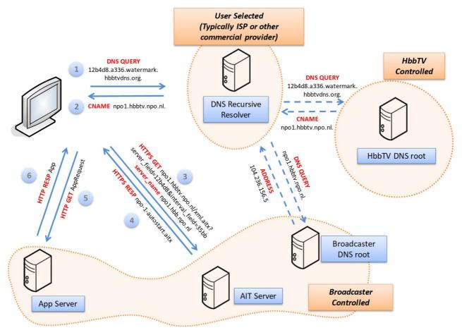
Figure 2: HbbTV<sup>®</sup> Application Discovery over Broadband in the presence of watermark information
