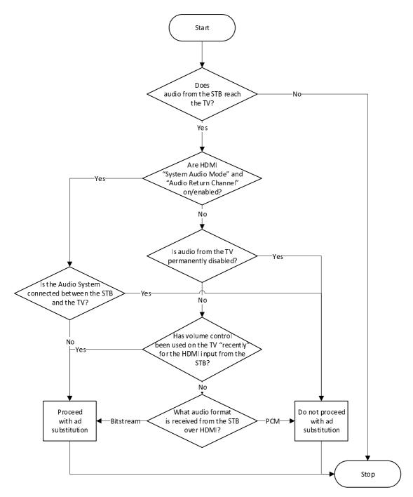
Figure D.1:Example audio configuration decision process
