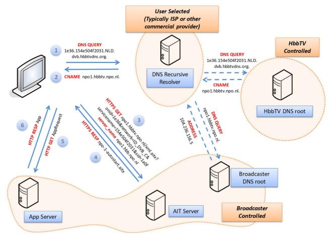
Figure 1: HbbTV® Application Discovery over Broadband in the presence of DVB Service Information
