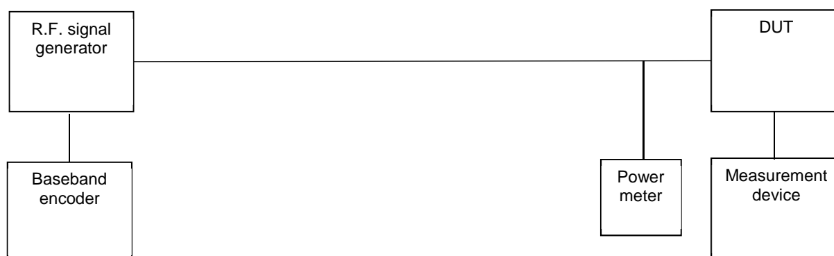
Figure 5: Conducted test set up for Gaussian sensitivity
