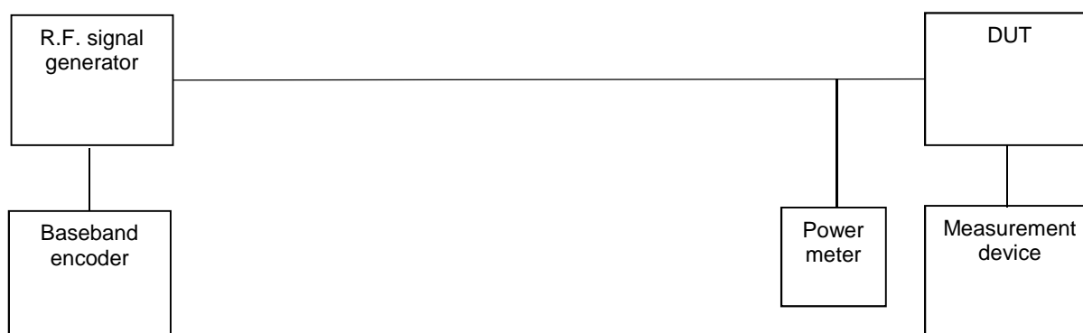
Figure 5: Conducted test set up for Gaussian sensitivity
