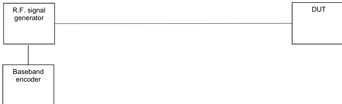
Figure 3: Test set up with one signal generator
