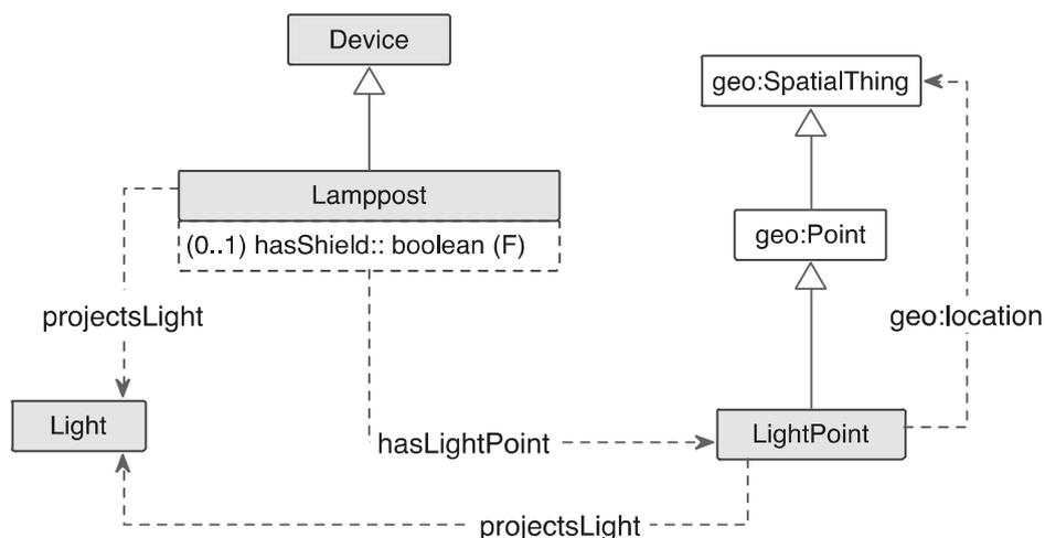
**Figure 8: Lamppost and light point model**
