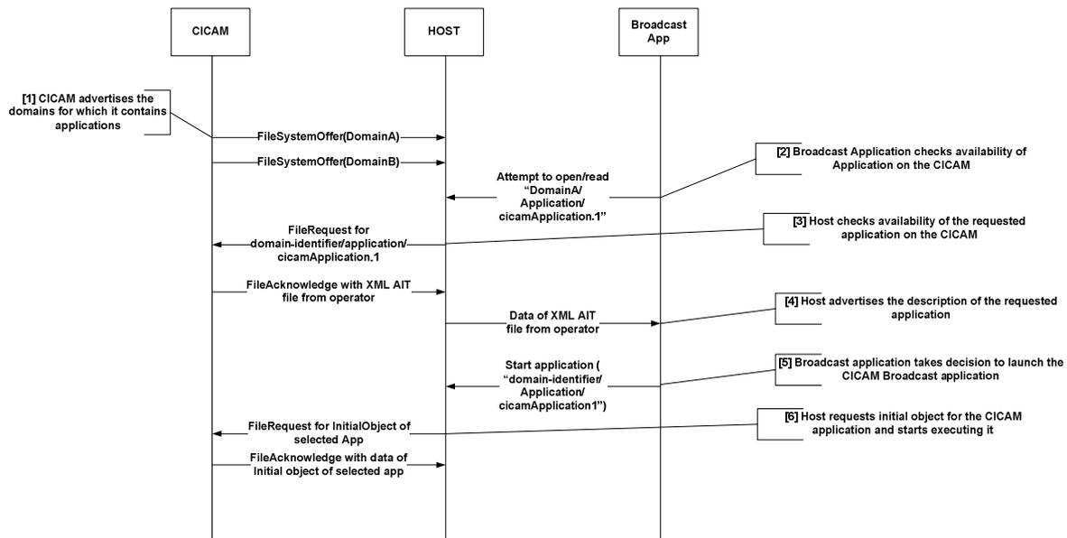
**Figure 24: Broadcast application launches CICAM broadcast application example**
