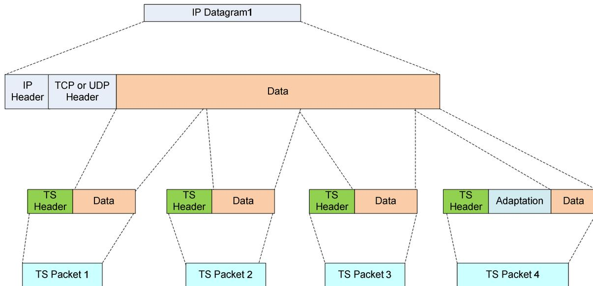
**Figure 21: Mapping of IP datagram to TS packets**
