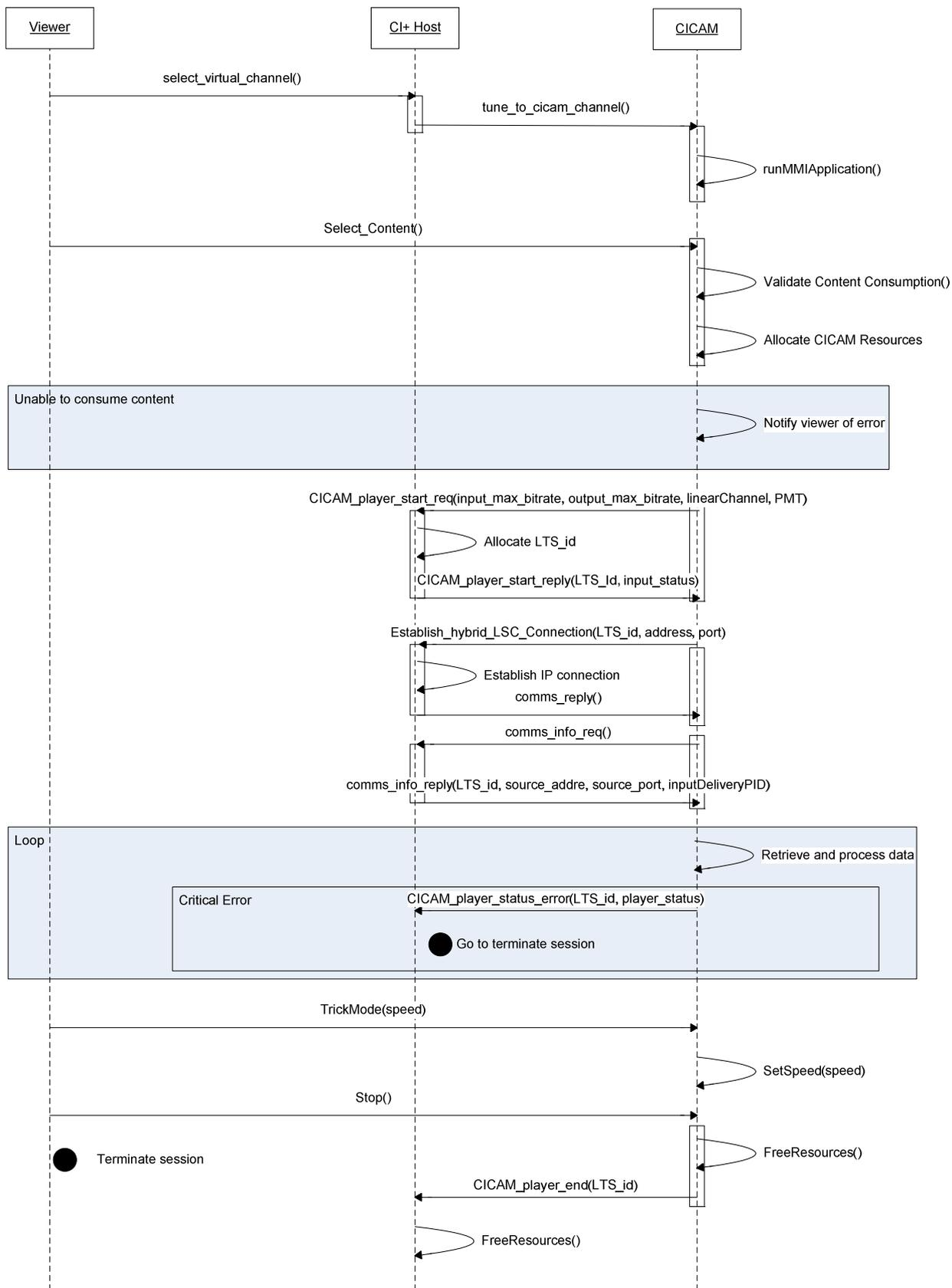
Figure 19: Example sequence diagram for CICAM-initiated playback
