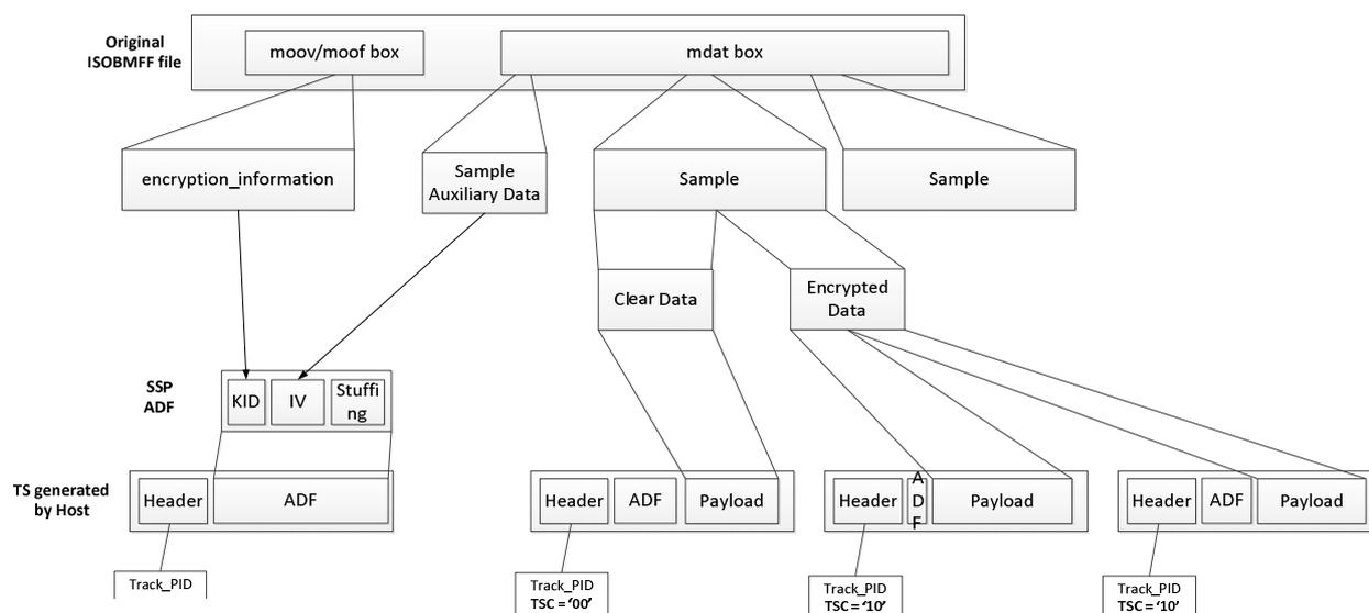
Figure 17: Encapsulation of ISOBMFF content into a TS
