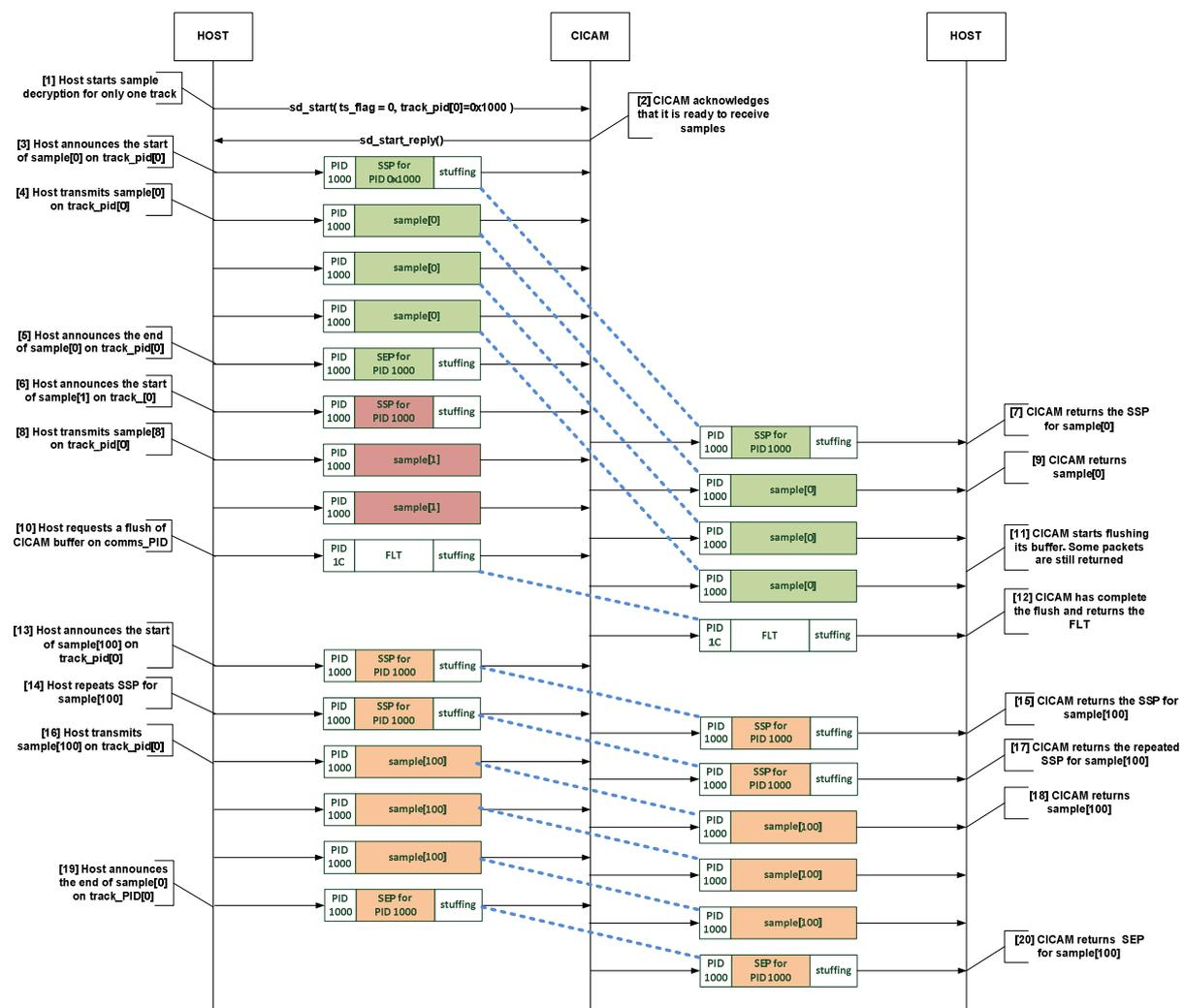
Figure 16: Example sequence with non-TS content buffer flush
