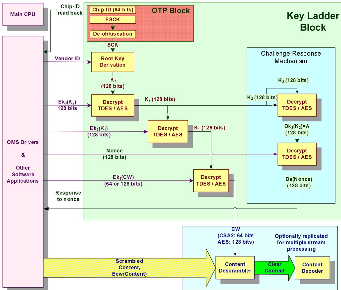
Figure 1: Key Ladder Functional Diagram
