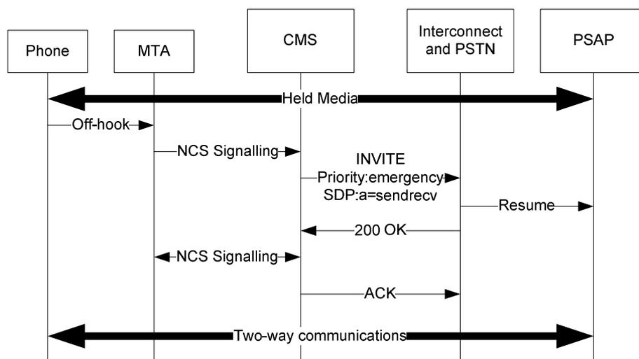
**Figure 12: Emergency Call; Network Hold Resume procedures**
