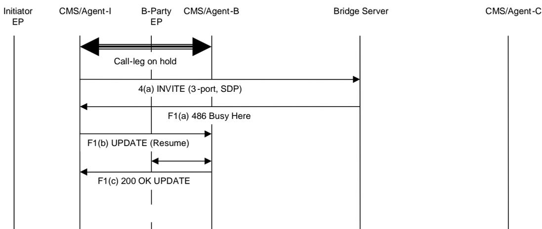
Figure 16: Failure ca- F1 - no free conference circuits
