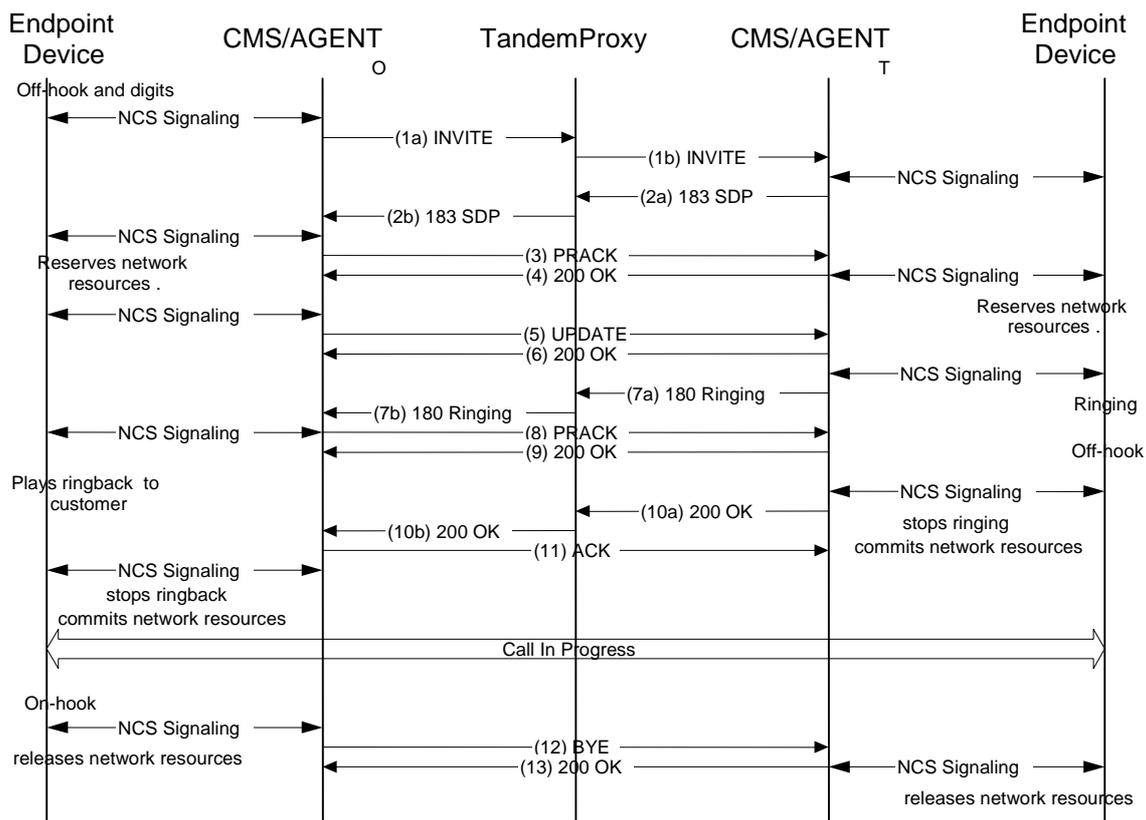
Figure 4: CMS - CMS Signaling Basic Call Flow
