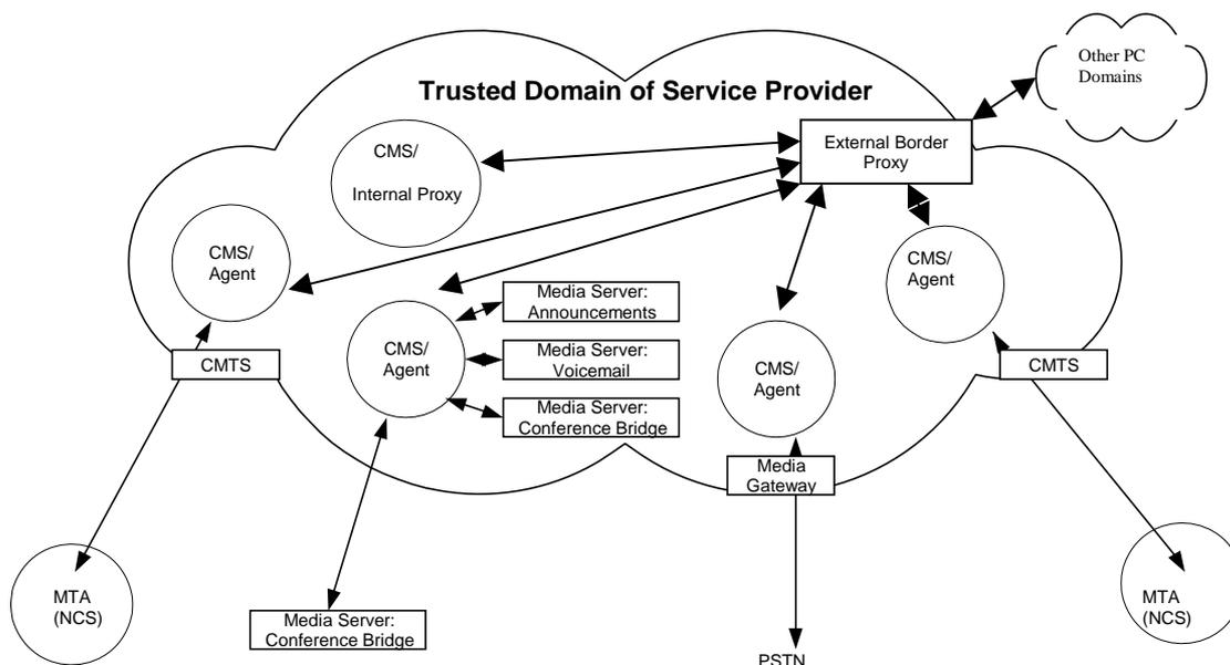
Figure 2: Trusted Domain of IP Cablecom Service Provider
