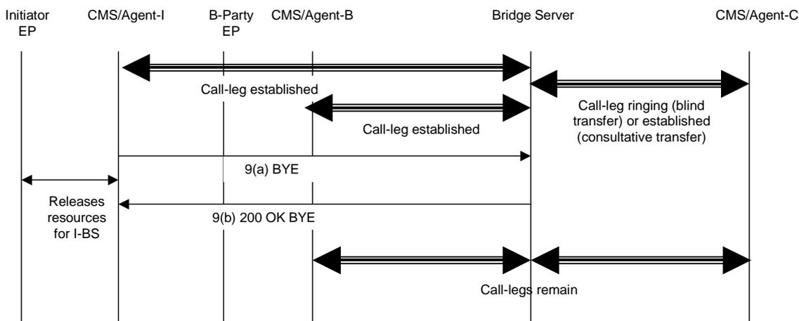
**Figure 21: Transfer completed, CMSI ends involvement in call**
