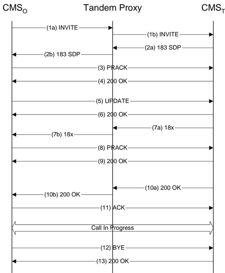
**Figure 10: CMS Messages for Basic Call Setup**
