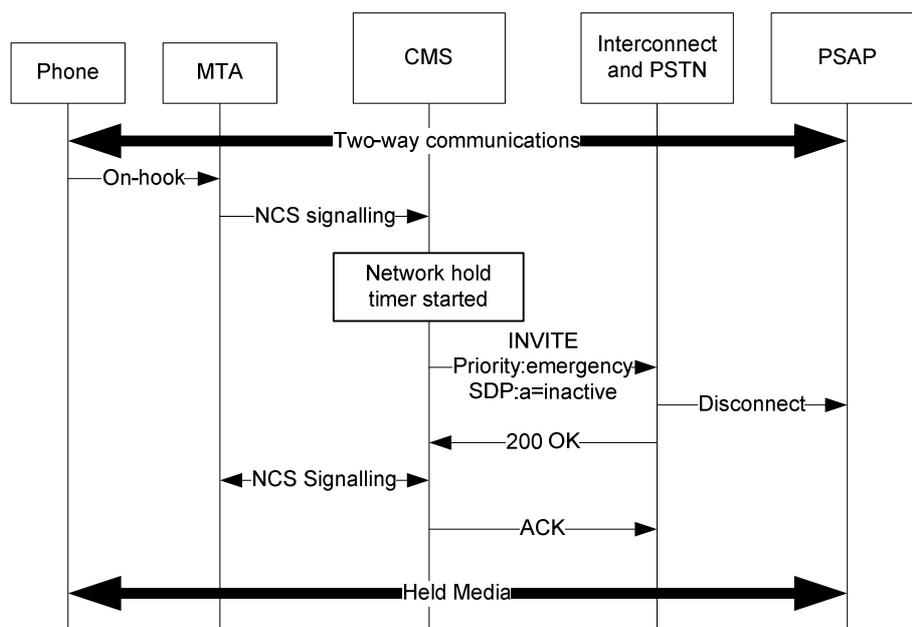
**Figure 11: Emergency Call; Network Hold Disconnect procedures**
