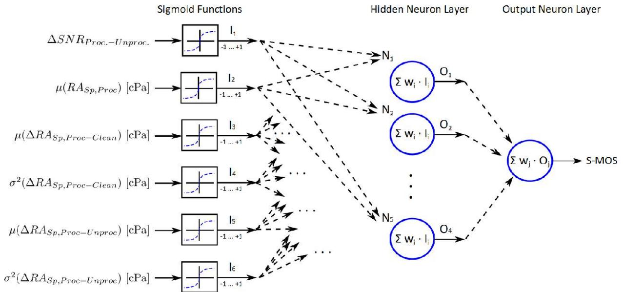
**Figure 1: Structure of neural network for S-MOS**
