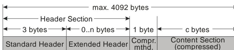
**Figure 7: JML object with compressed content section**
