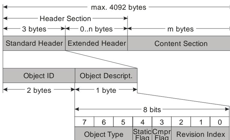
Figure 6: Components of a JML object
