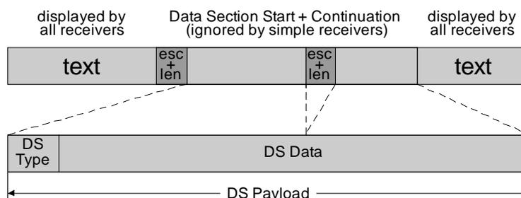
**Figure 8: Data sections and payload structure**
