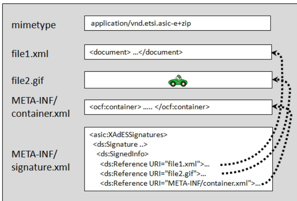
Figure 3: ASiC-E with XAdES and direct ds:reference usage
