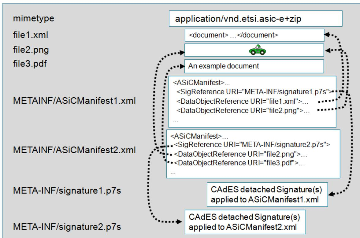
Figure 5: ASiC-E with CADES containing different signatures
