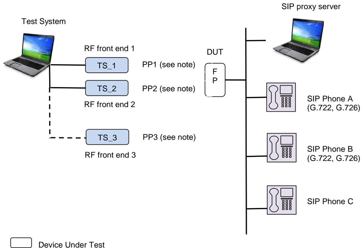
NOTE: PP1, PP2 and PP3 behave either as a NG PP, a legacy GAP PP, or a headset PP according to test case.
