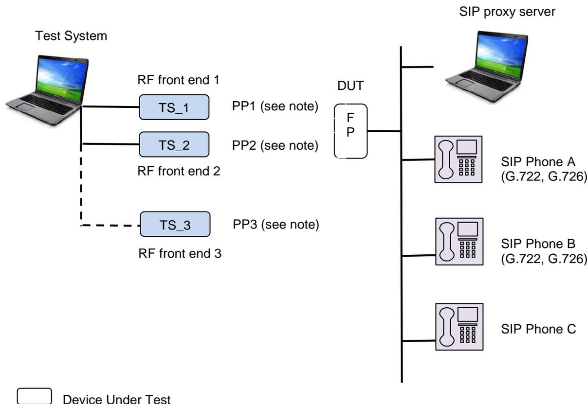
NOTE: PP1, PP2 and PP3 behave either as a NG PP, a legacy GAP PP, or a headset PP according to test case.
