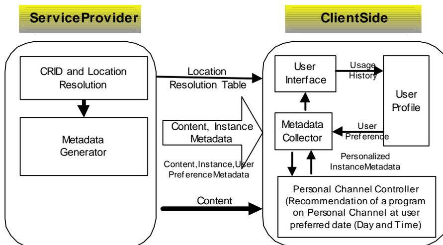
Figure 14: Interaction between Service Provider and Client
