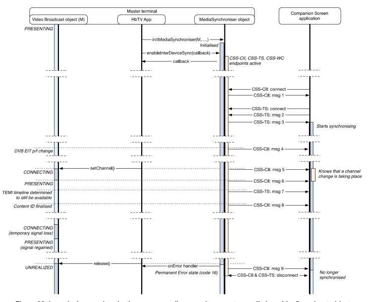
Figure 32: Inter-device synchronization sequence diagram where master media is a video/broadcast object
