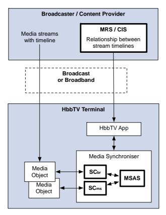
Figure 21: Basic mapping of media synchronization architecture for multi-stream synchronization
