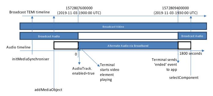
Figure M.1: Example of alternate audio track for a single broadast TV programme
