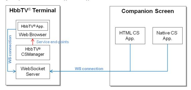
Figure 35: Architecture for application to application communication
