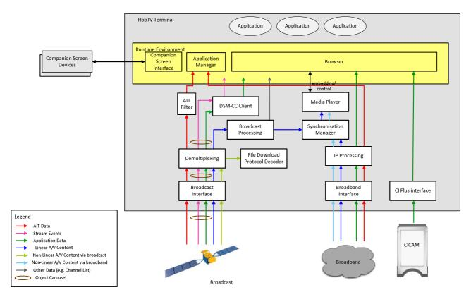
Figure 2: Functional components of a hybrid terminal
