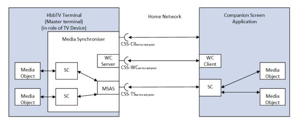
Figure 25: Relationship between the HbbTV<sup>®</sup> MediaSynchroniser and MSAS, SC, WC Server and WC Client elementary functions and protocol service endpoints
