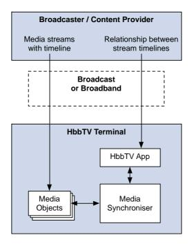
Figure 20: Relationship between MediaSynchroniser object and  $\mbox{HbbTV}^{\mbox{\scriptsize (B)}}$  application for multi-stream synchronization
