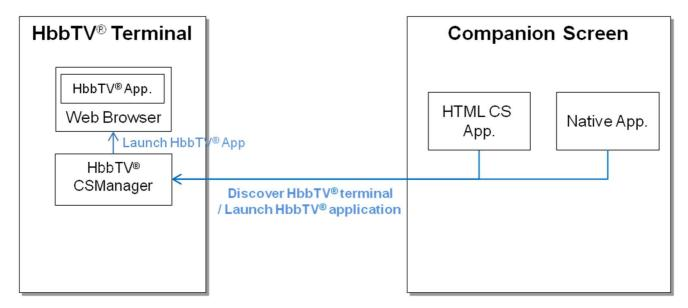
Figure 36: Architecture for remotely launching HbbTV® applications
