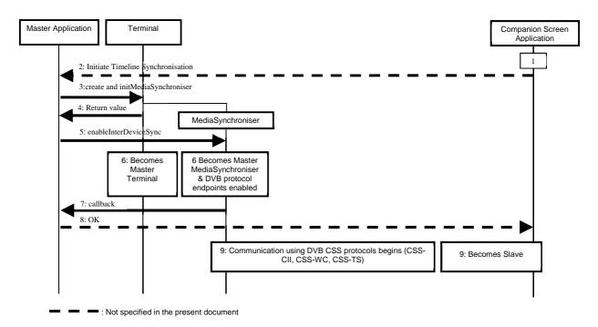
Figure 27: Initiation of inter-device timeline synchronization
