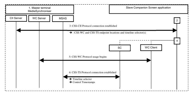
Figure 28: Protocol interactions for inter-device timeline synchronization
