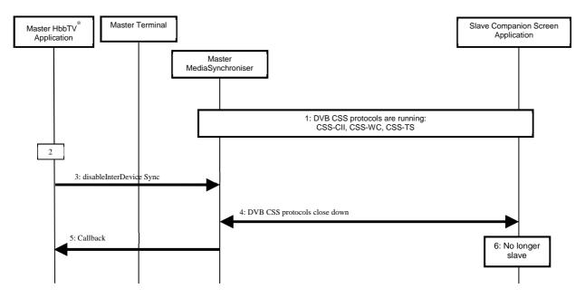
Figure 29: Termination of inter-device timeline synchronization
