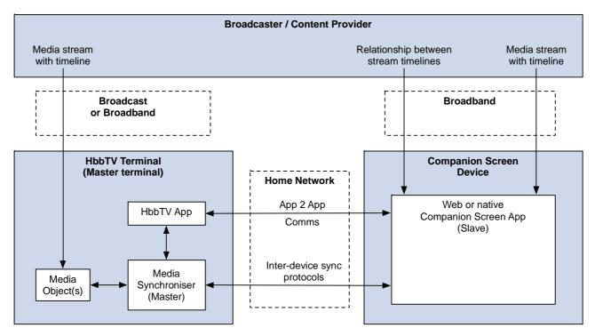
Figure 22: Relationship between MediaSynchroniser object and  $HbbTV^{\otimes}$  application for inter-device synchronization with a CSA
