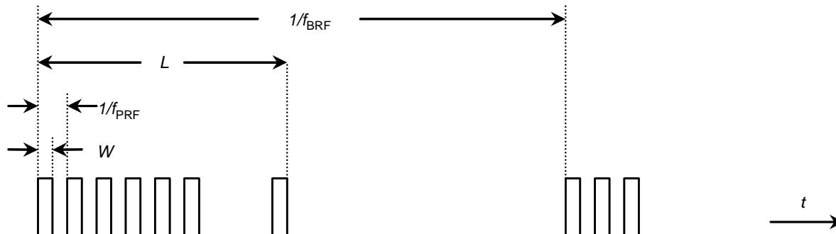
Figure D.4: General structure of the bursts for DAA radio location test transmissions
