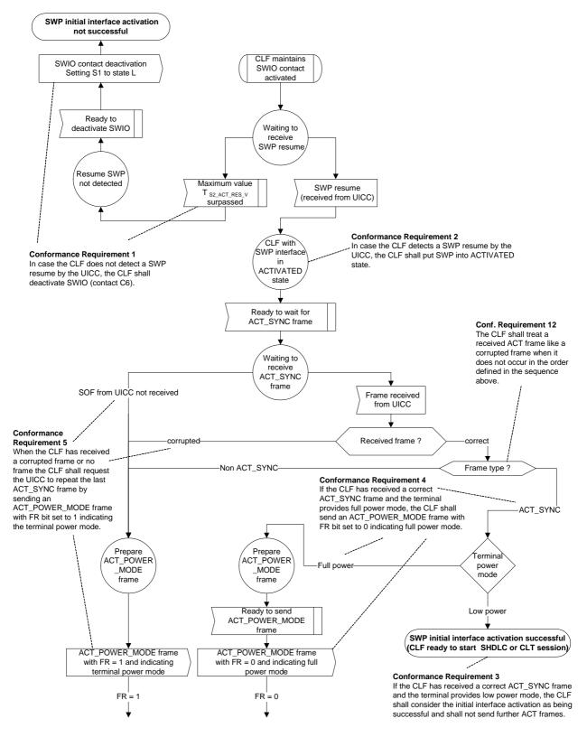
Figure A.2.1: Initial SWP interface activation, part 1
