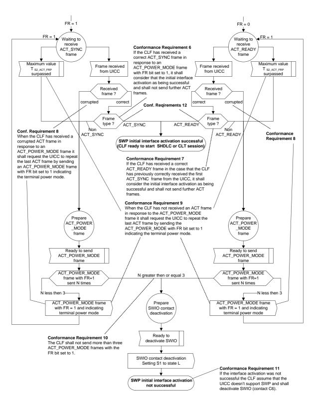
Figure A.2.2: Initial SWP interface activation, part 2
