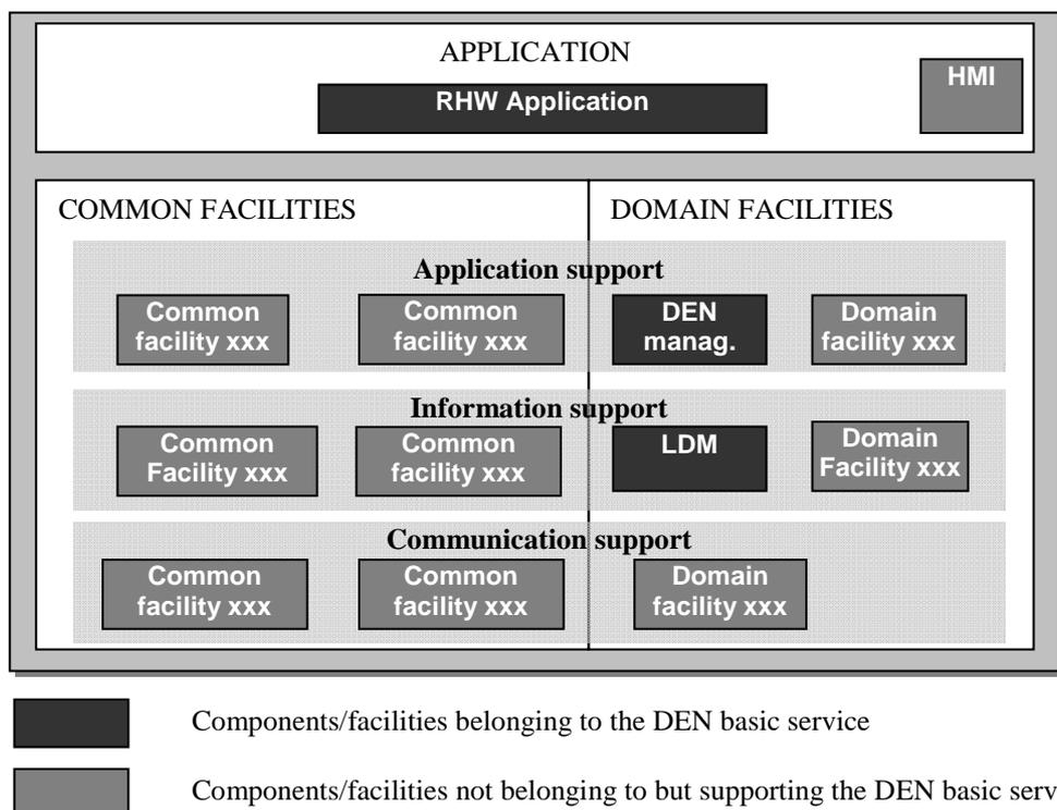
**Figure 1: DEN basic service components**
