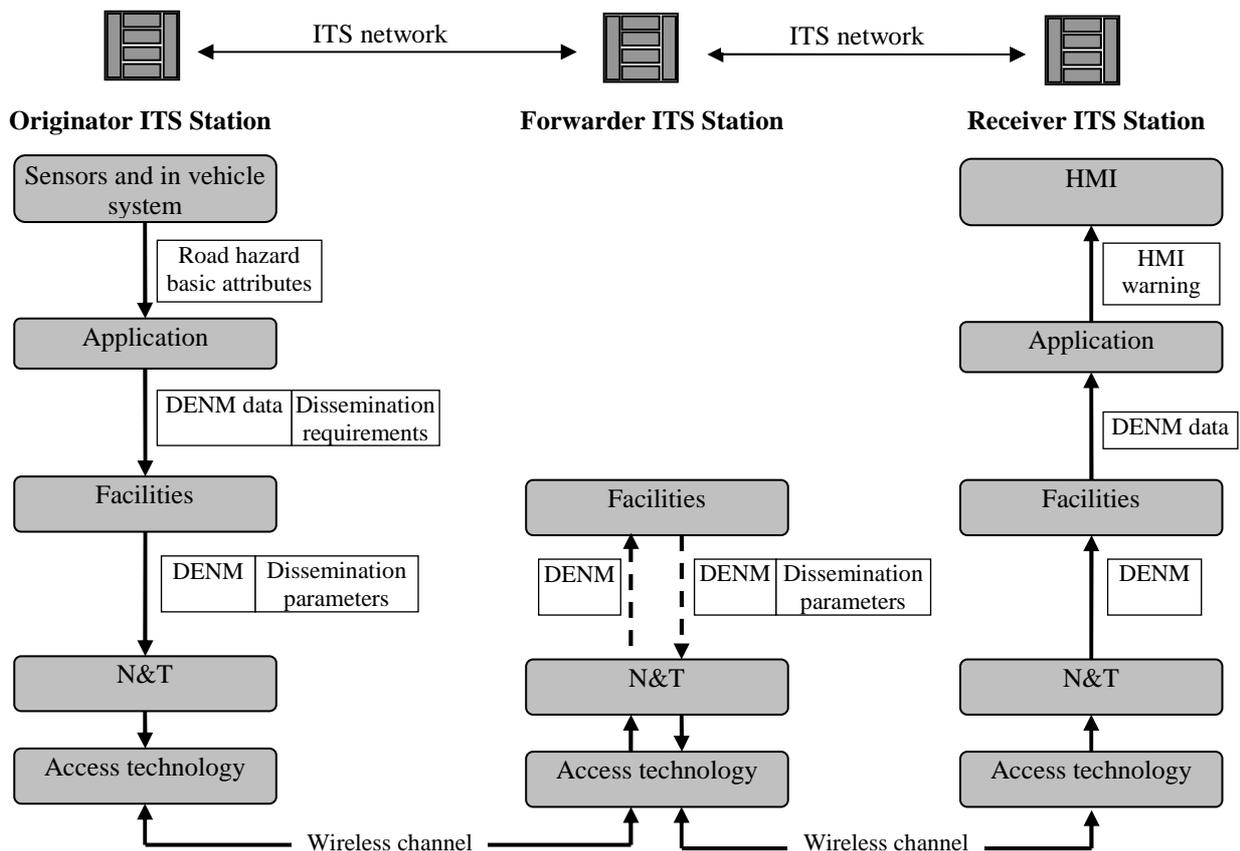
Figure C.1: General inter layer dataflow for road hazard warning application and DENM
