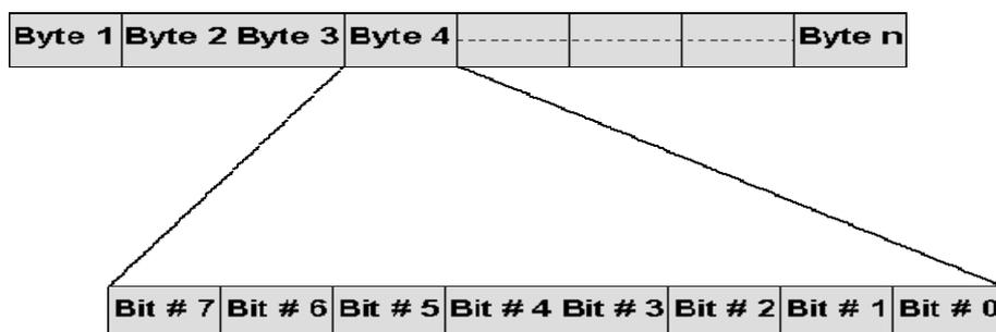
Figure 5: Bits and bytes in DENM
