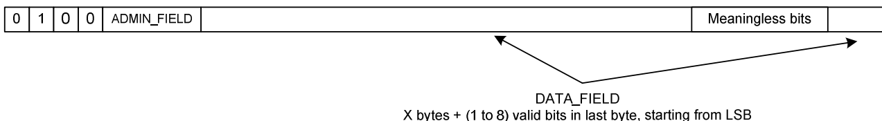
CLT LPDU with DATA_FIELD „byte aligned“ structured
