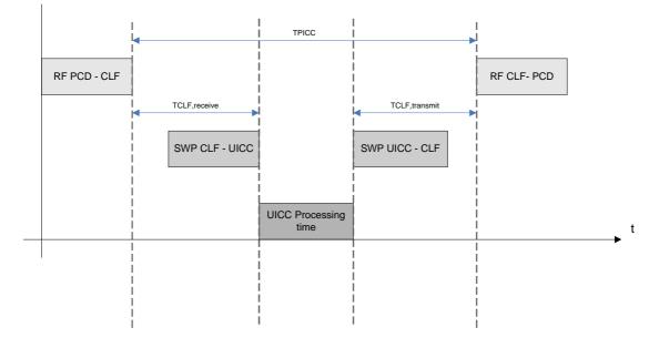
NOTE: SWP CLF-UICC and SWP UICC-CLF represent the time taken to transmit the data over SWP and are included in the T<sub>CLF.receive</sub> and T<sub>CLF.transmit</sub> times.
