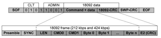
Figure 11.3: Type F structured CLT frame
