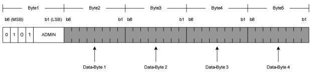
Figure 11.4: Type F byte alignment in CLT frame
