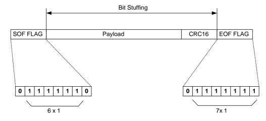
Figure 9.2 illustrates the format of a frame sent from the master to the slave.
