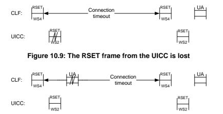
Figure 10.10: The UA from the CLF is lost and the connection timeout allows restarting the link configuration
