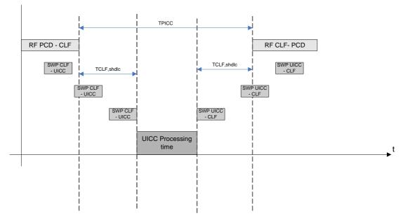
Figure 12.5: SHDLC transmission timings
