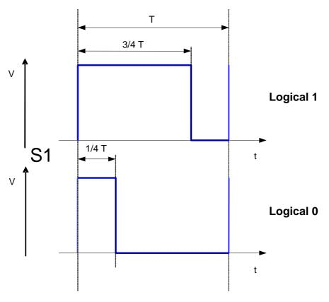
Figure 8.1: Bit-coding of S1
