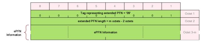
Figure 7: Overall structure of ePFN tag
