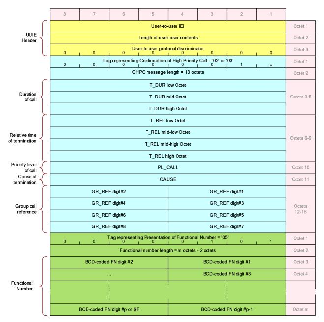
Figure 12: CHPC "Format A" tag layout
