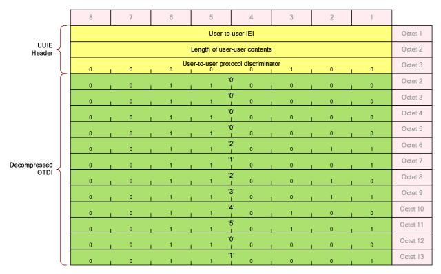
Figure 19: Example of expansion of compressed OTDI
