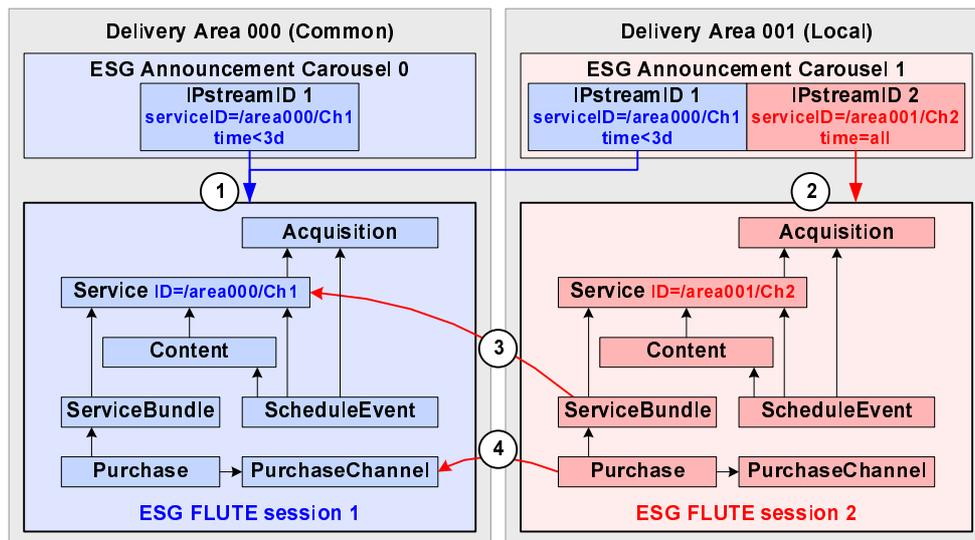
Figure 2: ESG instantiation mechanisms 1, 2, 3 and 4
