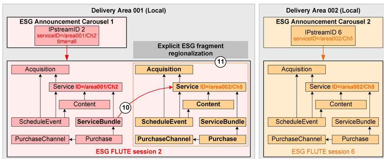
Figure 6: ESG instantiation mechanism 11 (not recommended)
