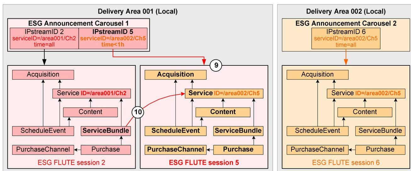
Figure 5: ESG instantiation mechanisms 9 and 10
