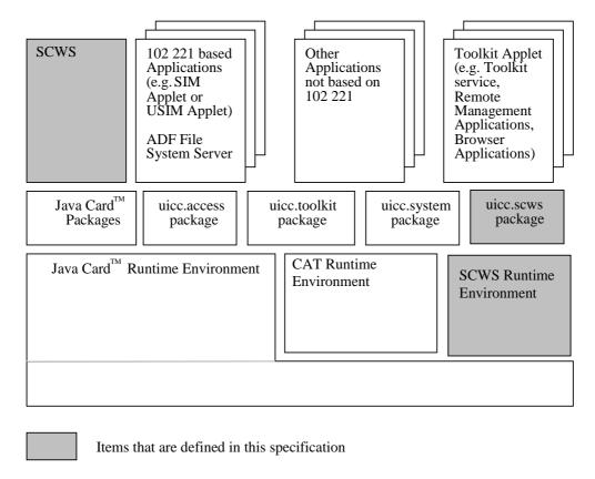
**Smartcard Webserver (SCWS):** handles Http request as defined by OMA in [3] and [4] and provides a mechanism to the Applet for the registration.
