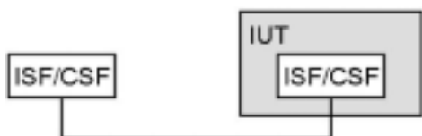
Figure A.6: Configuration CF_dPMR_ISF/CSF_01_C
