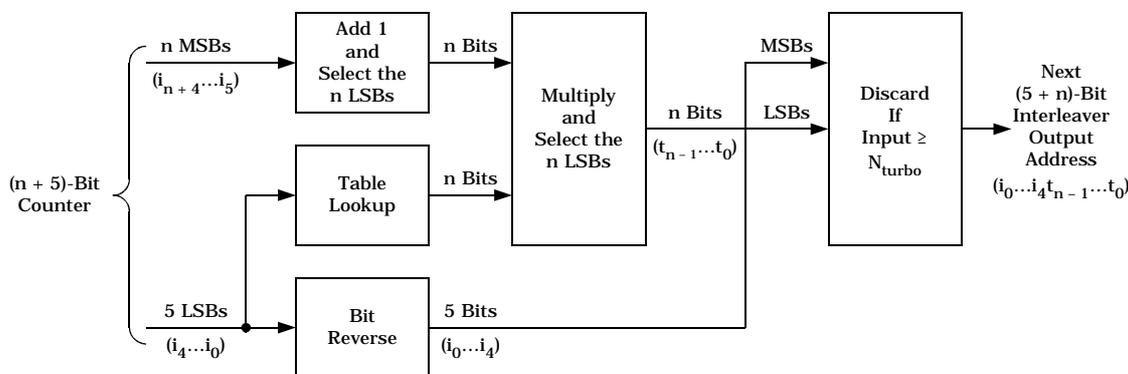
Figure 5: Turbo interleaver output address calculation procedure
