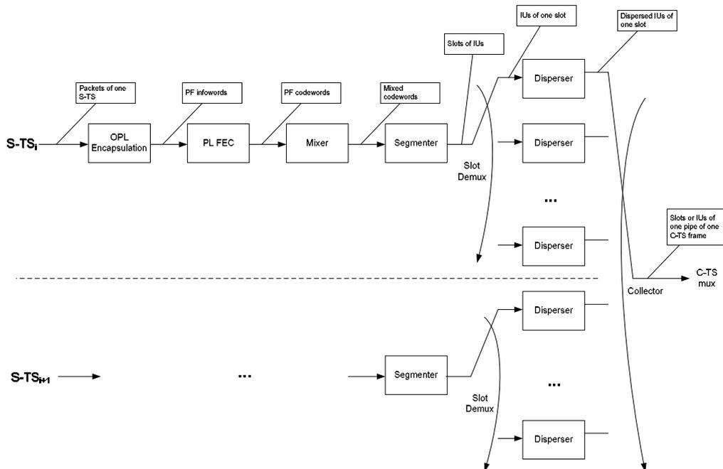
**Figure 2: Definition of the different blocks involved in the OPL processing**
