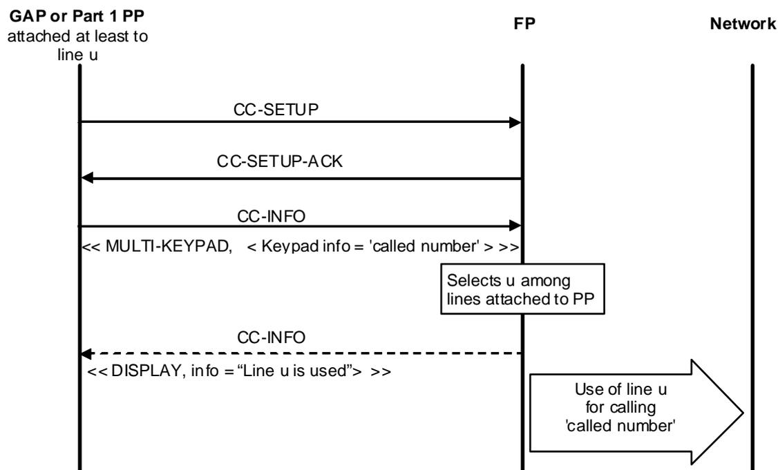
**Figure 41: Backward compatible FP managed line selection**
