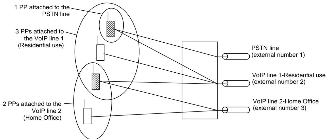
**Figure 51: Example of a multiple line configuration with 3 lines (with attachments)
