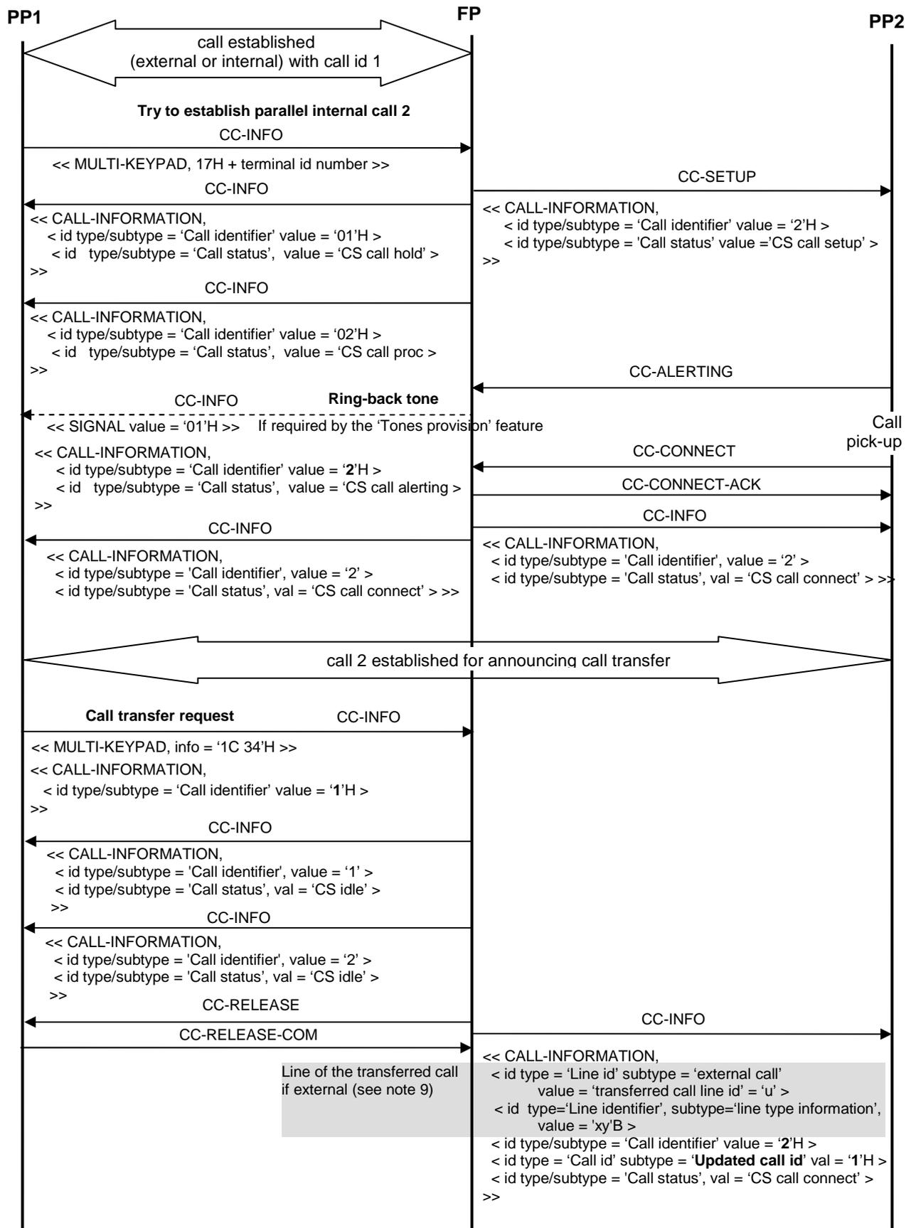
Figure 17: Announced call transfer (example with internal target PP2):
