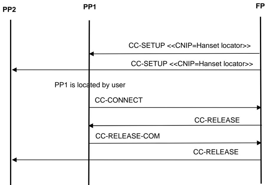
**Figure 85: Handset locator example where PP1 is located**
