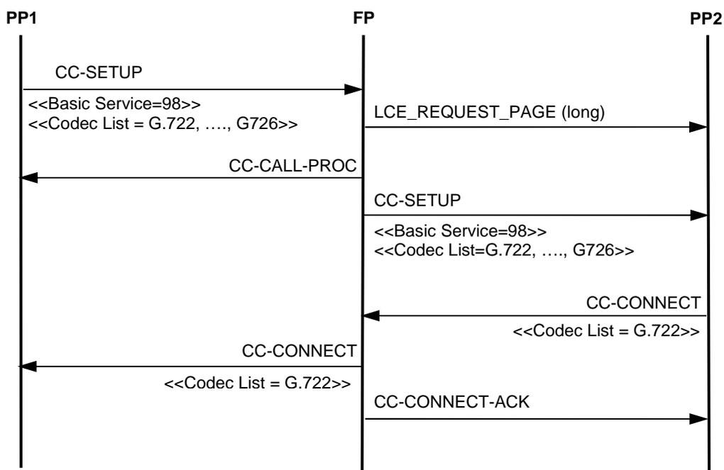
**Figure 28: Internal call with codec list at call setup**
