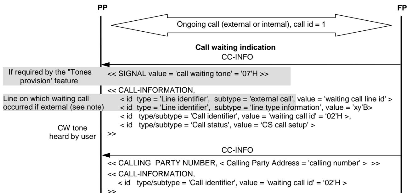
NOTE: The line identifier indicates to the PP on which line the waiting call occurred and also indicates the 'line type information' of this line (if external).
