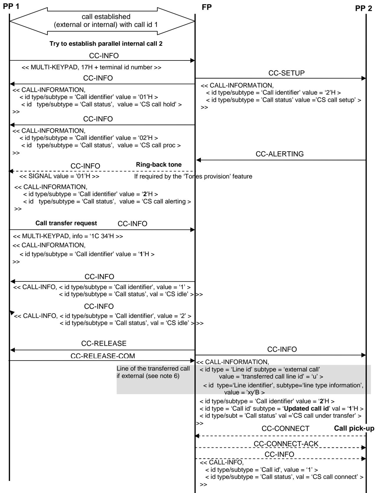
Figure 18: Unannounced call transfer (example with internal target PP2):
