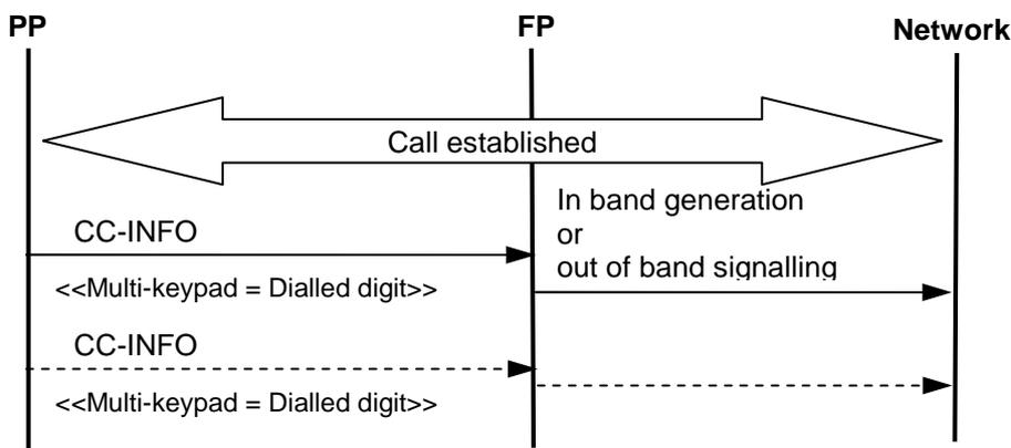
Figure 67: Sending DTMF when a call is established
