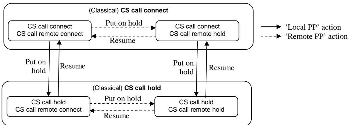
NOTE: The 'CS call remote connect' and 'CS call remote hold' call statuses concern the remote status of the call and are only a way to improve the user interface of the local PP. They do not interfere in any way with the local call statuses of the call, as shown in this figure.
