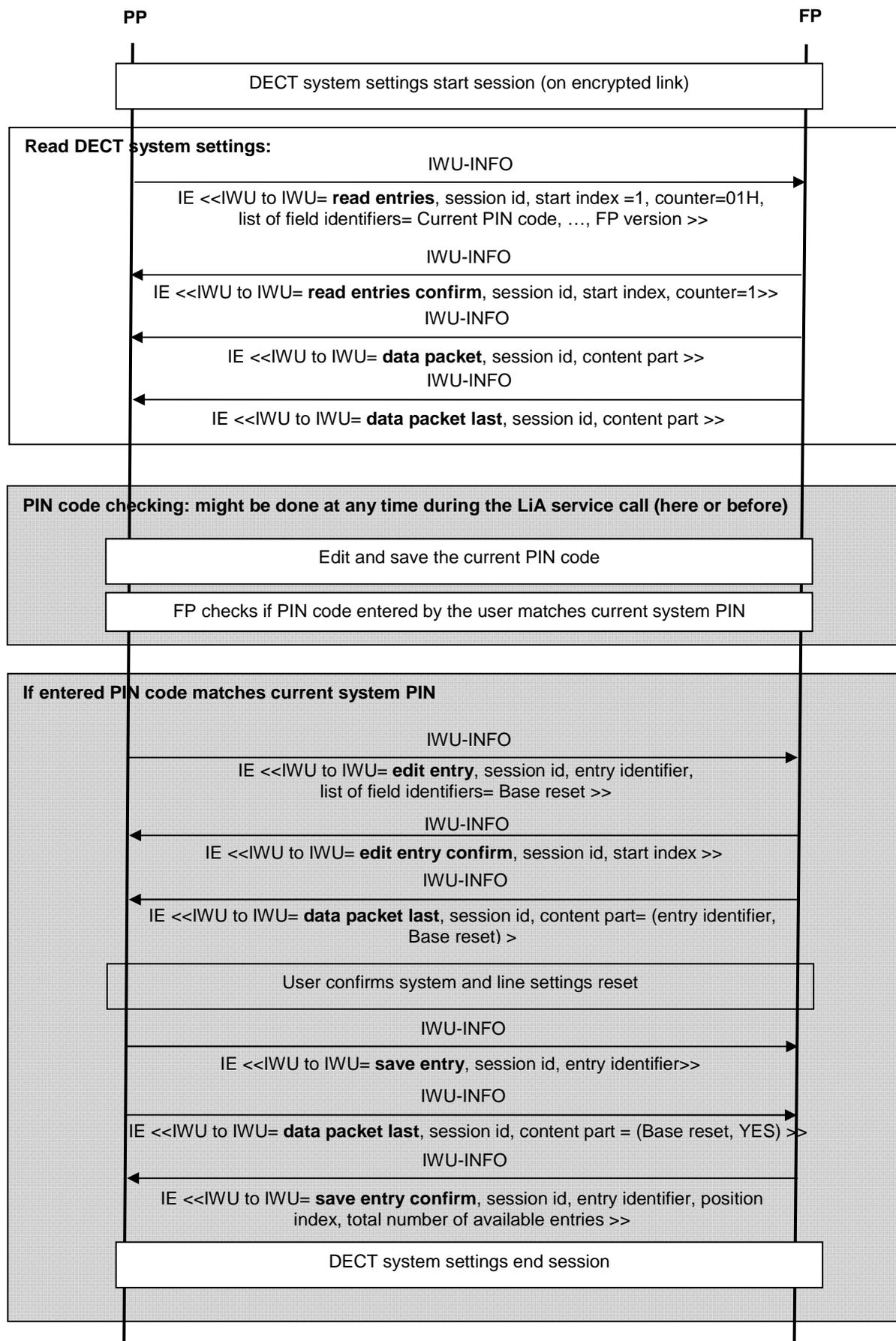
Figure C.33: Resetting the base (PIN protected field)
