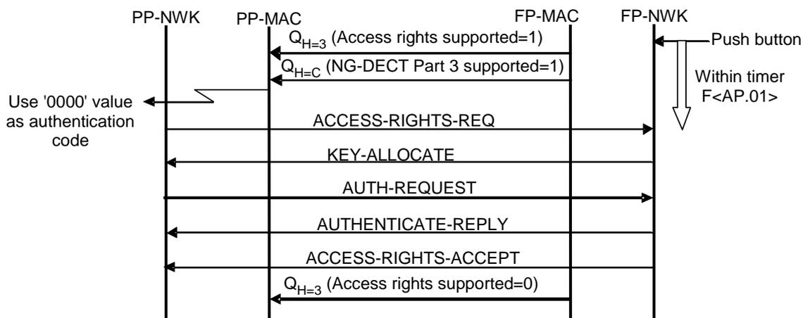
Figure 82: Easy pairing when PIN is set to default '0000' value
