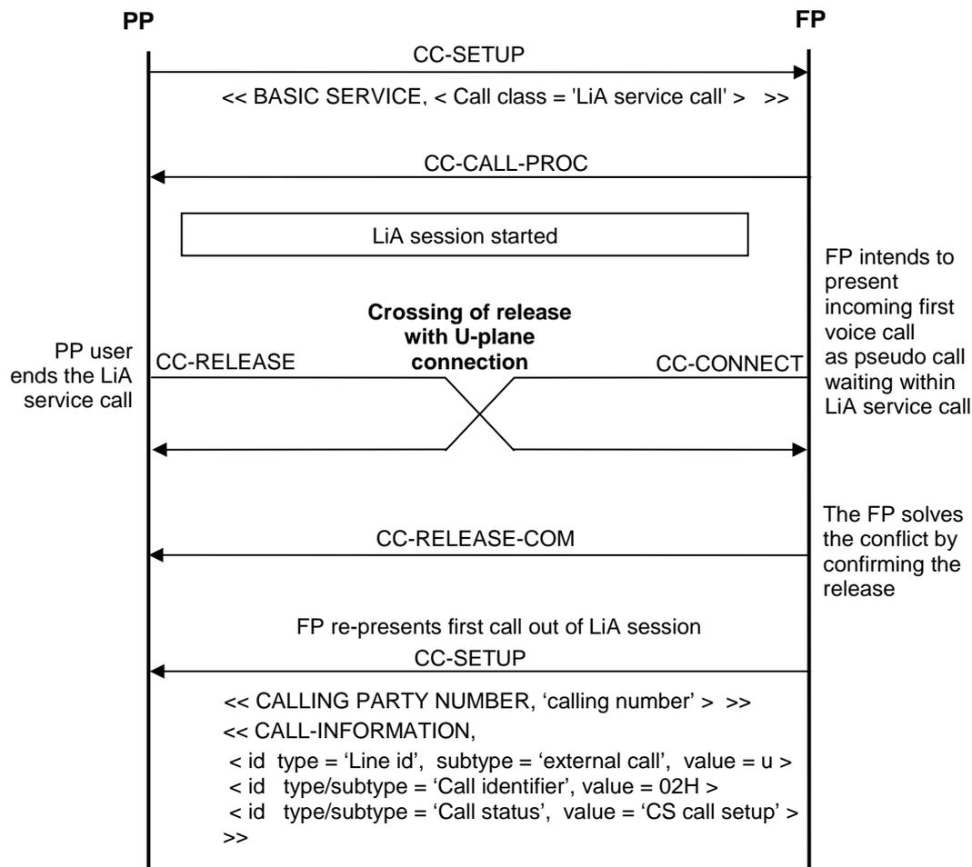
Figure 59a: {CC-CONNECT} and {CC-RELEASE} crossing use case
