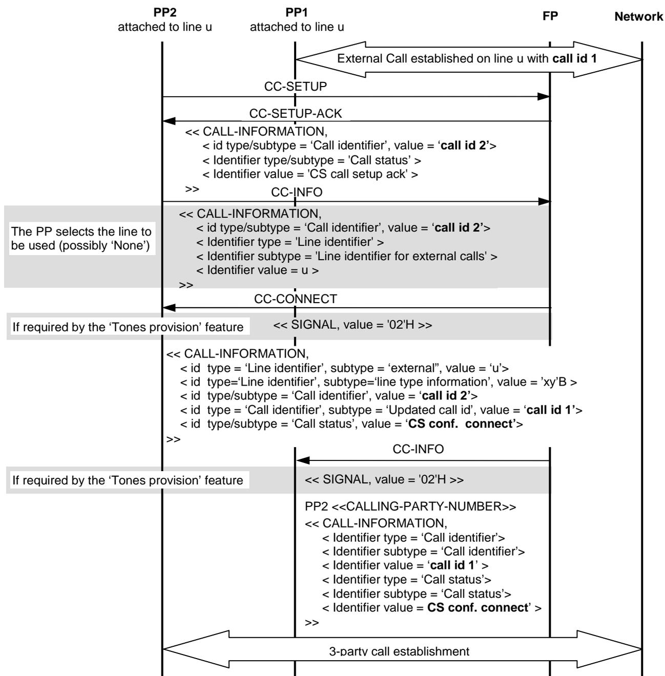
**Figure 25: Implicit intrusion call with PP line selection in a {CC-INFO}**
