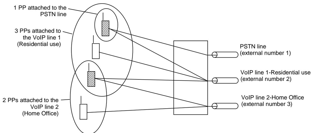
**Figure 52: A multiple-call line with three simultaneous calls**
