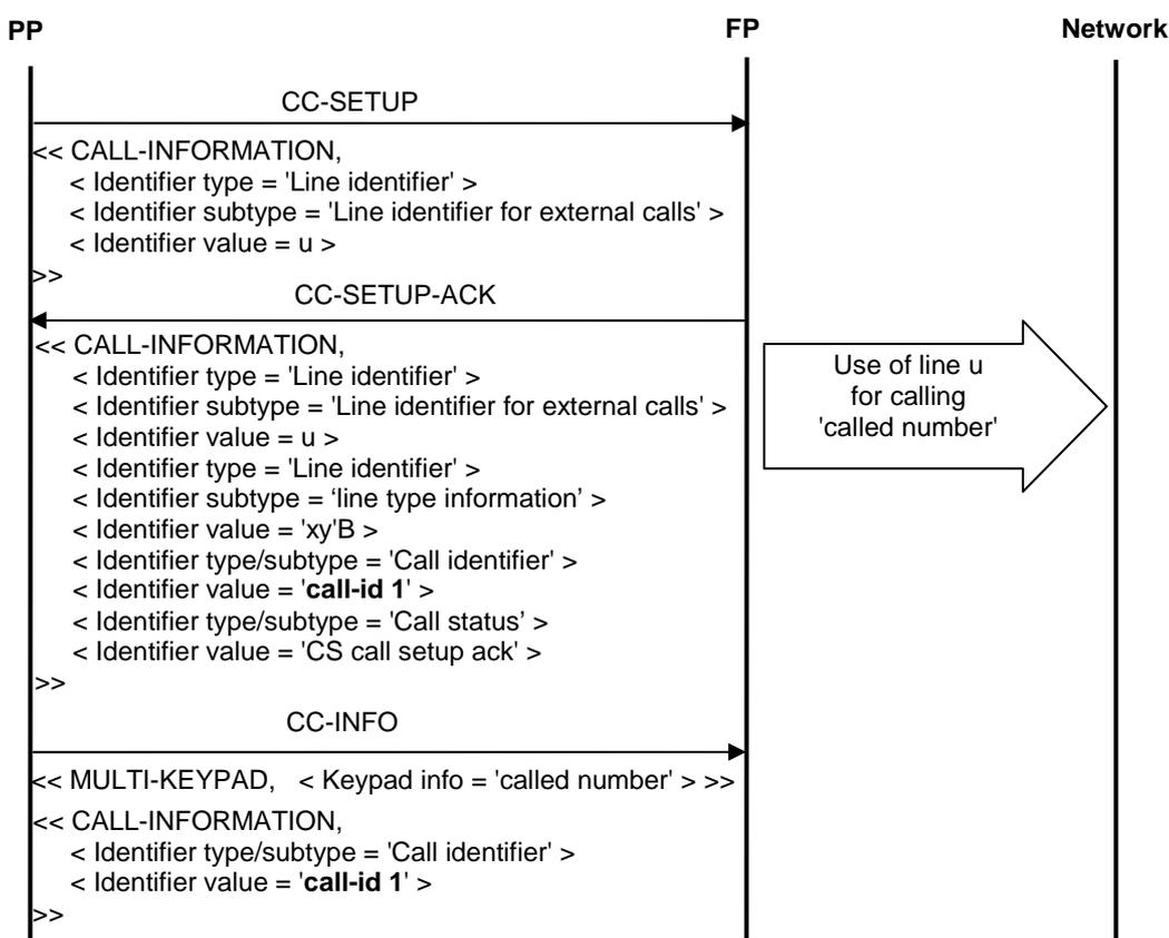
**Figure C.2: Line identification by PP using <<CALL-INFORMATION>>**
