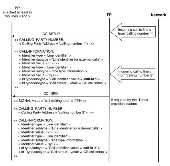
Figure C.15: Incoming parallel calls: two simultaneous incoming calls on two different lines
