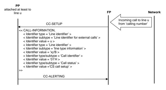
Figure 42: Line identification for a first external incoming call
