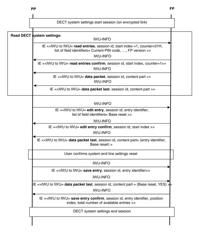
Figure C.32: Resetting the base
