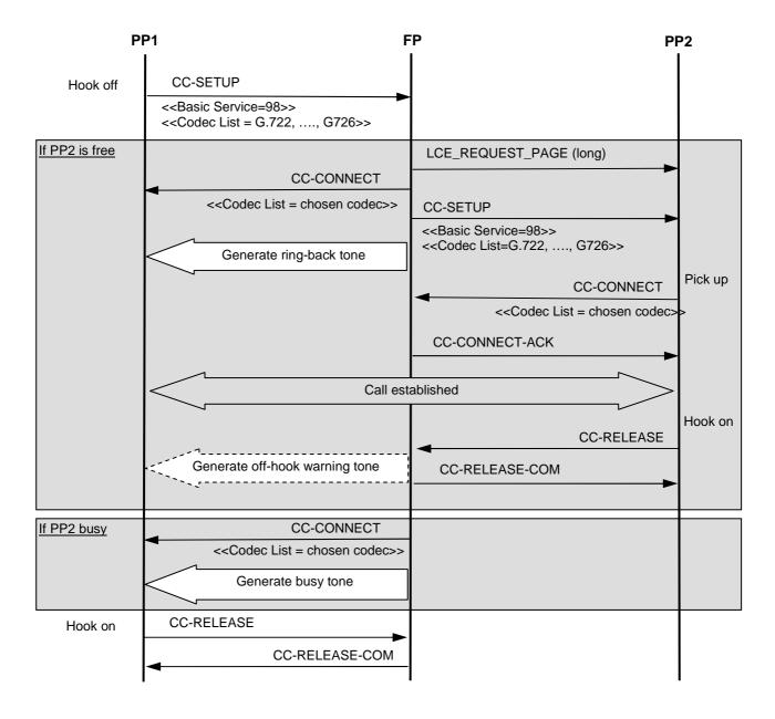
Figure 76: FP provides tones during Internal call using {CC-CONNECT}
