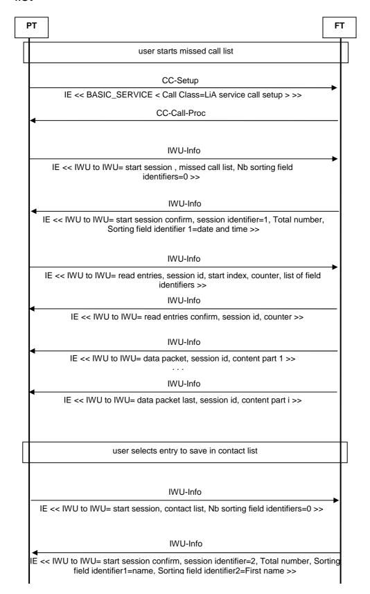
Figure C.19: List access use case: transfer number from missed call list to contact list (1/2)
