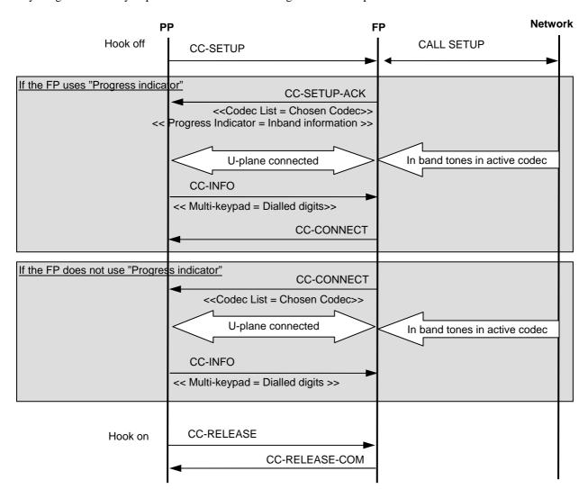
Figure 77: Network provides tones during PSTN external call
