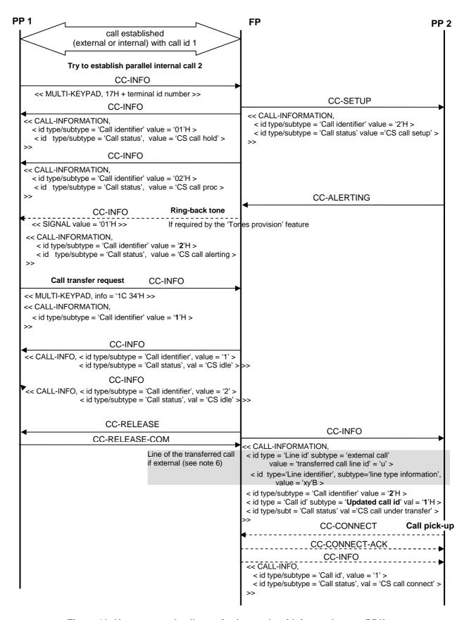
Figure 18: Unannounced call transfer (example with internal target PP2):
