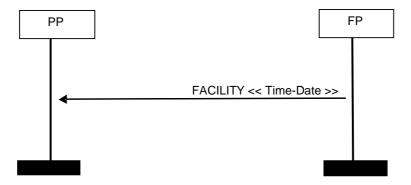
Figure B.7: Date-time synchronization during existing connection
