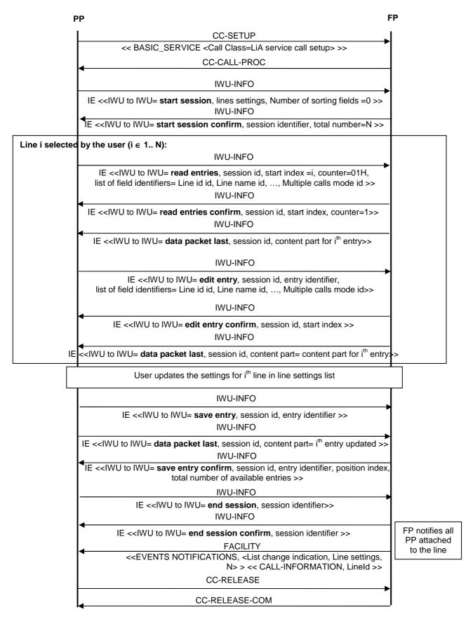
Figure C.34: Changing the settings of a line (use case 1)
