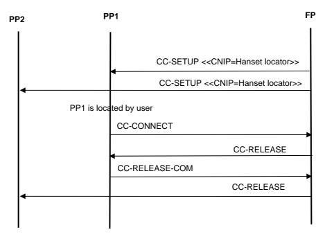
Figure 85: Handset locator example where PP1 is located
