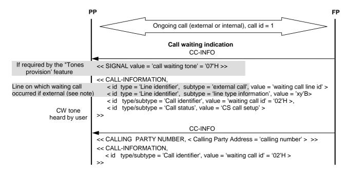
NOTE: The line identifier indicates to the PP on which line the waiting call occurred and also indicates the 'line type information' of this line (if external).
