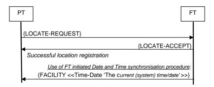
Figure 79: After successful PT location registration, the FP systematically uses the "FT initiated Date and Time synchronisation procedure
