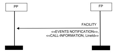
Figure B.2: Event notification during existing connection
