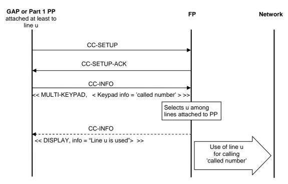
Figure 41: Backward compatible FP managed line selection
