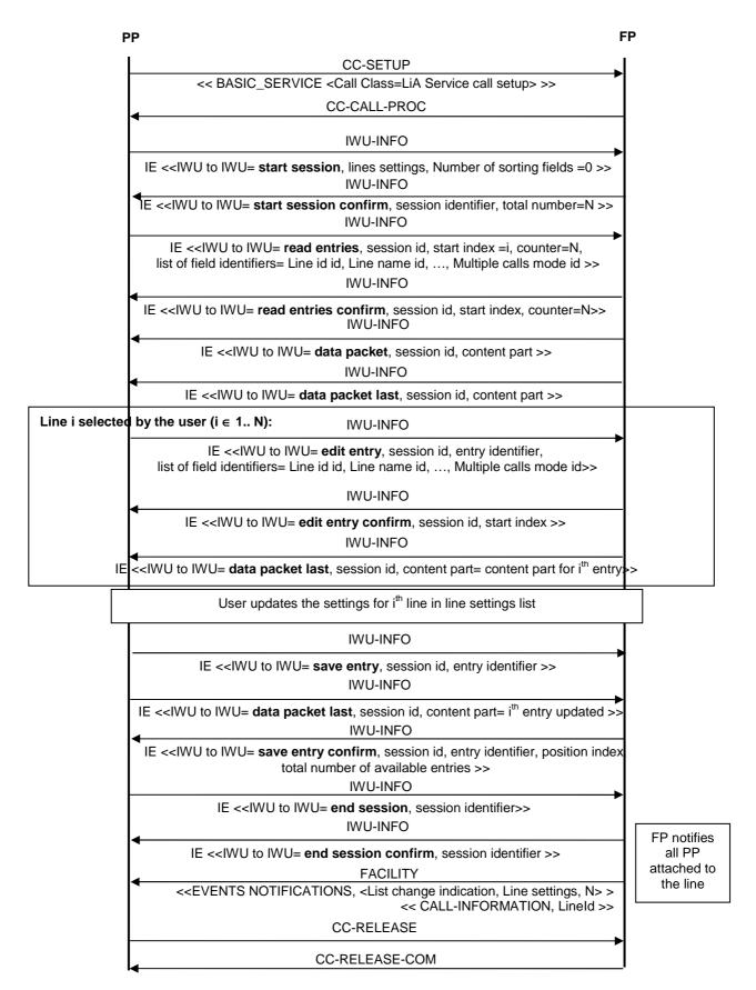
Figure C.35: Changing the settings of a line (use case 2)
