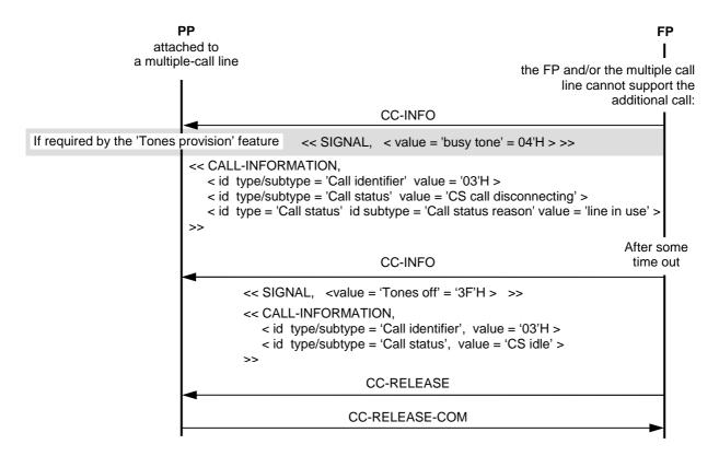
Figure 53: Busy system or line notification for call with defined call-id=3
