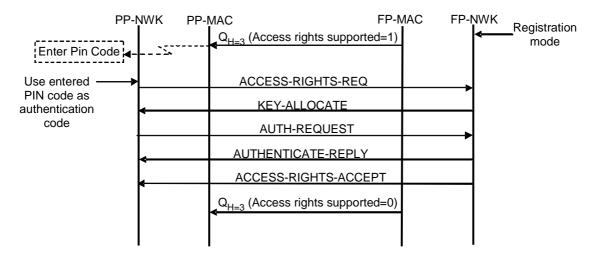
Figure 81: Easy PIN code registration mode
