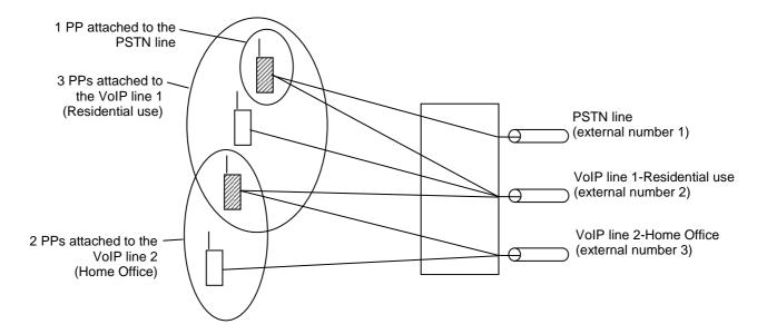
Figure 52: A multiple-call line with three simultaneous calls
