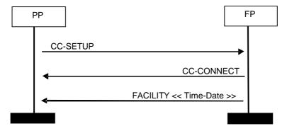
Figure B.9: Date-time synchronization using call connection
