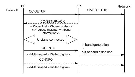
Figure 66: Using overlap sending and DTMF to establish a call
