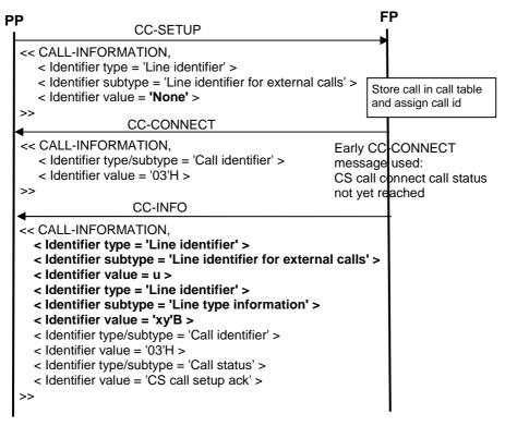
Figure 40: Example of use with an early {CC-CONNECT} implementation
