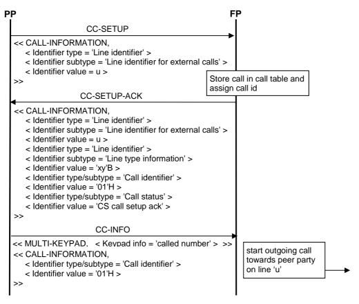
Figure 33: Line identification in {CC-SETUP}
