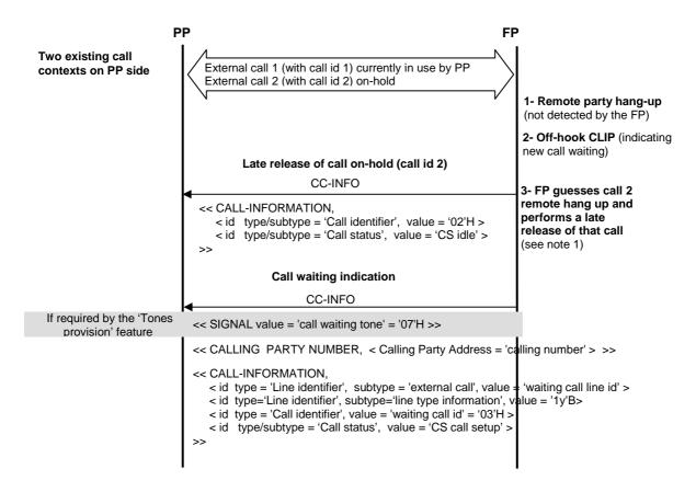
Figure C.39: Late release of call on-hold following call waiting indication
