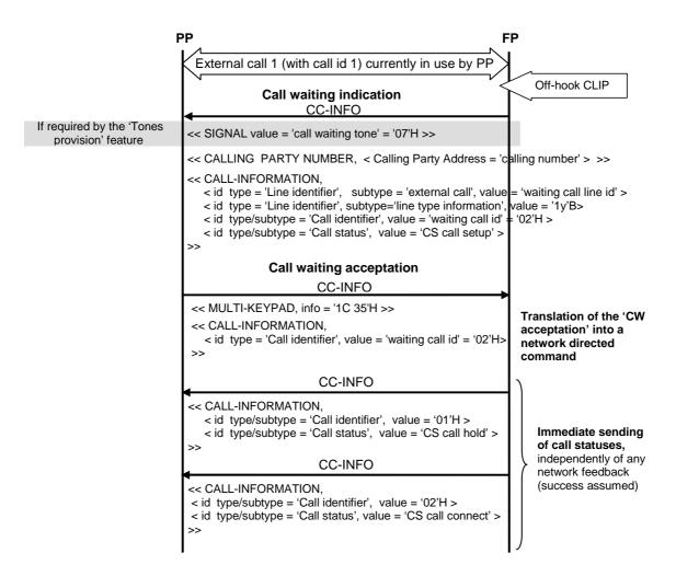
Figure 29: Call waiting acceptation within an 'off-hook CLIP enabled DCIBS' line
