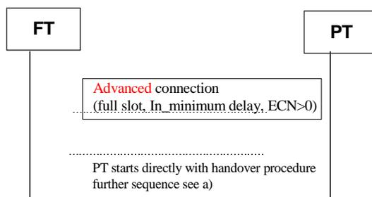
**Figure D.37: Successful PT initiated connection modification (full slot I<sub>N</sub>\_minimum\_delay -> long slot I<sub>N</sub>\_minimum\_delay); initial connection is advanced**
