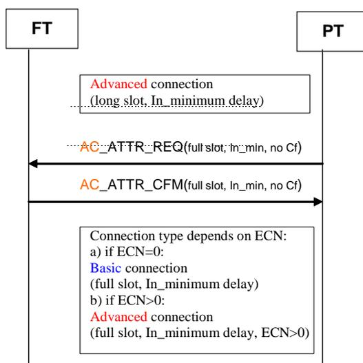
**Figure D.41: PT initiated connection modification (long slot I<sub>N</sub>\_minimum\_delay -> full slot I<sub>N</sub>\_minimum delay)**
