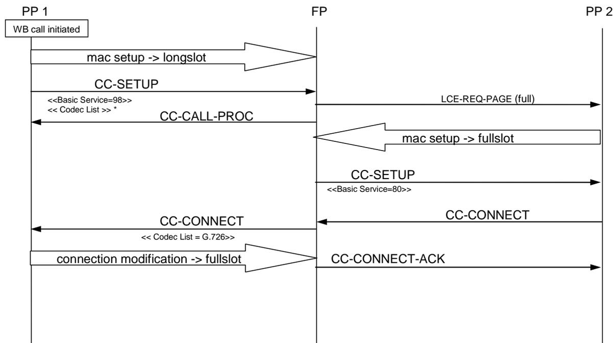
Figure D.16: Intercom Call with Interworking: WB Handset -> NB Handset
