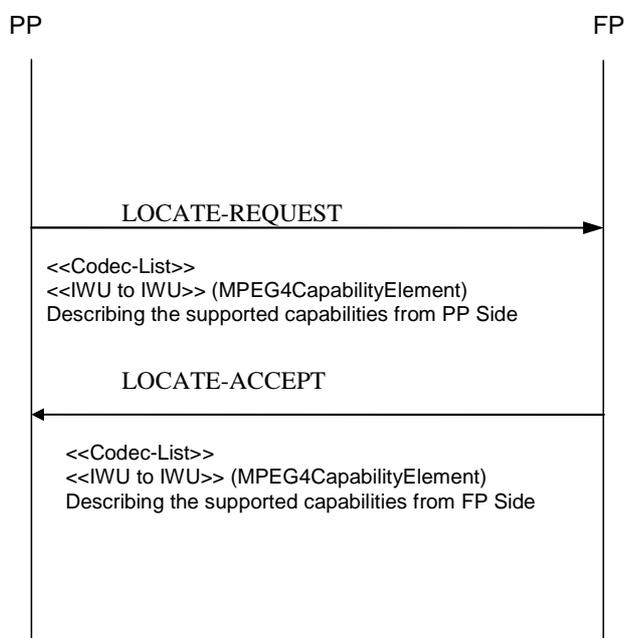
**Figure D.43: Transmitting non default configuration using <<LOCATE-REQUEST>>, <<LOCATE-ACCEPT>> Message**
