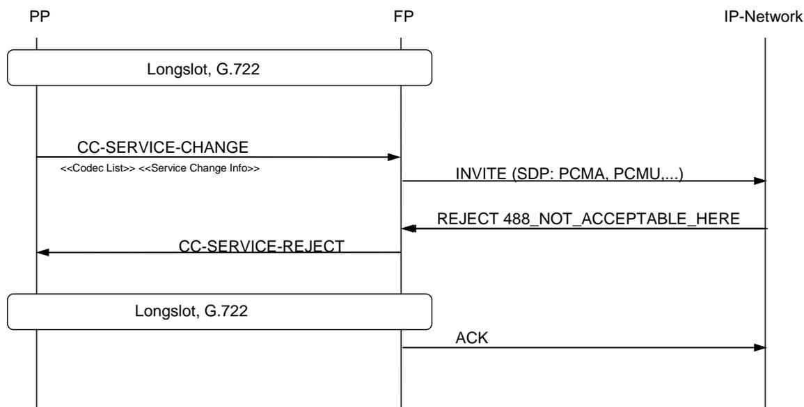
**Figure D.13: Service Change from Wideband ITU-T Recommendation G.722 [17] to Narrowband; PP initiated; IP Network does not accept Narrowband Codec**
