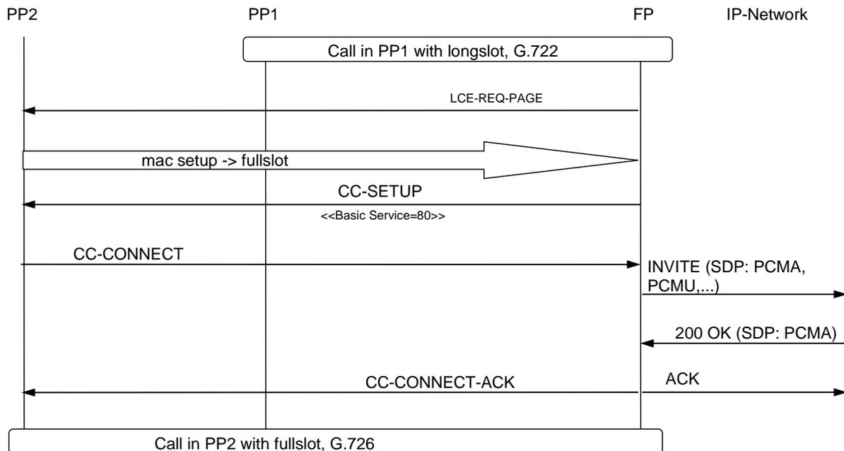
Figure D.19: Internal Call transfer from a NG PP to a PP which does not support wideband
