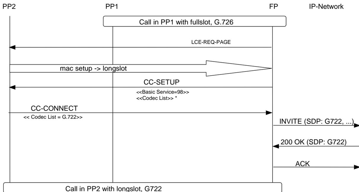
Figure D.20: Internal Call transfer, NB -> WB
