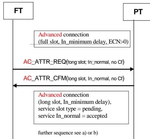
**Figure D.32: Successful FT initiated connection modification (full slot  $I_{N\_minimum\_delay}$  -> long slot  $I_{N\_normal}$  delay): initial connection is advanced**
