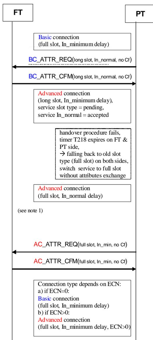
NOTE 1: After falling back to old slot type the initiating side starts a connection modification attributes exchange to leave the undefined/undesired state.
