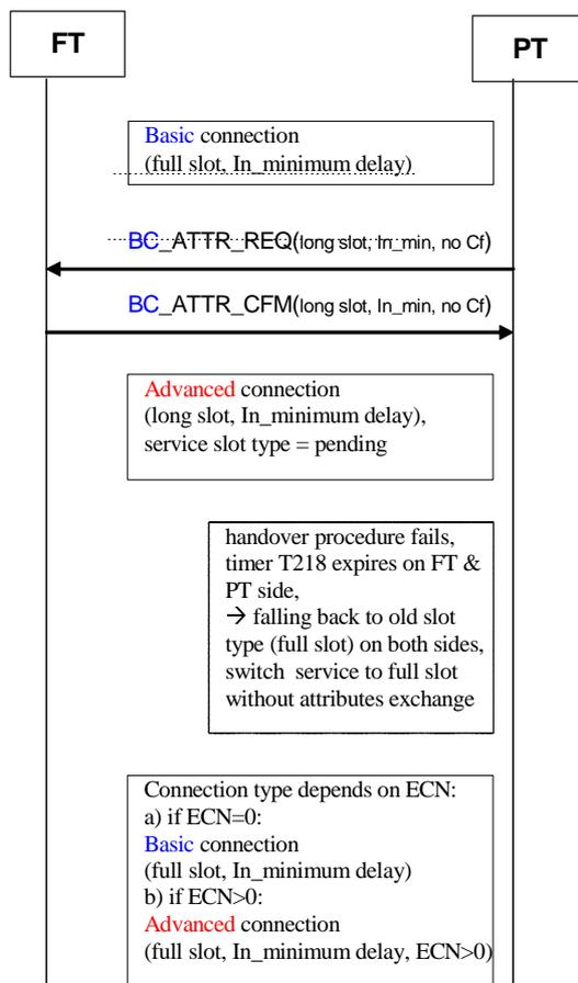
**Figure D.36: PT initiated connection modification failed (full slot I<sub>N</sub>\_minimum\_delay -> long slot I<sub>N</sub>\_minimum\_delay)**
