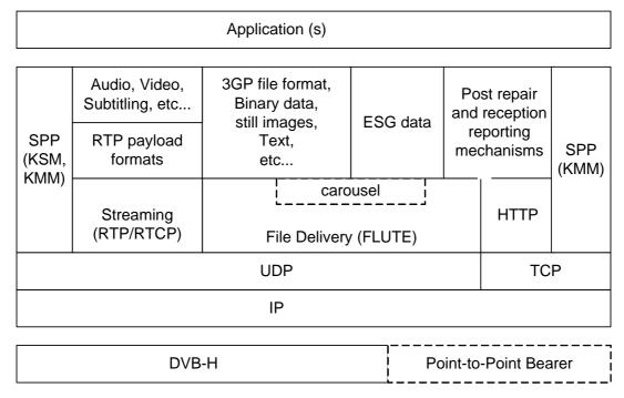
Figure 1: Baseline IPDC Protocol Stack for content delivery
