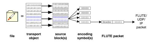
Figure A.1: Constructing of FLUTE Packets
