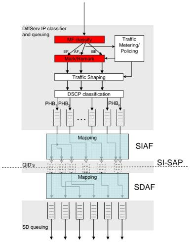
Figure 5: User-Plane detailed architecture of a DiffServ-aware ST
