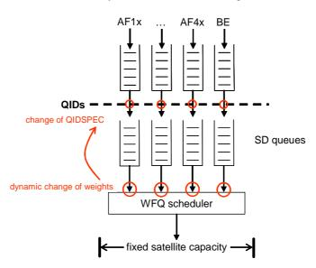
Figure 8: QID-to-SD static mapping with dynamic change of the QIDSPEC
