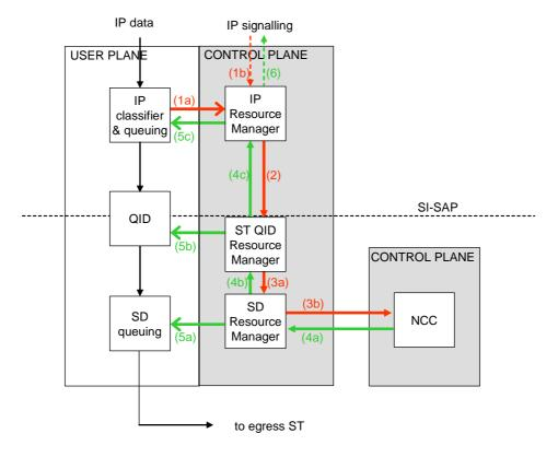
Figure 6: Control-Plane operations of a DiffServ-aware ST
