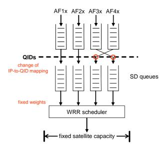
Figure 9: QID-to-SD static mapping with dynamic change of the IP-to-QID mapping
