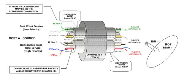
Figure A.2 shows the relationship between IP flows, C2P connections, PIDs and Channel-ids.
