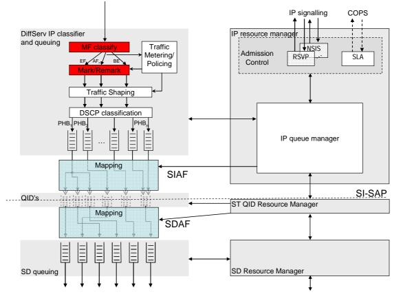
Figure 7: Detailed architecture of an ingress DiffServ-aware ST
