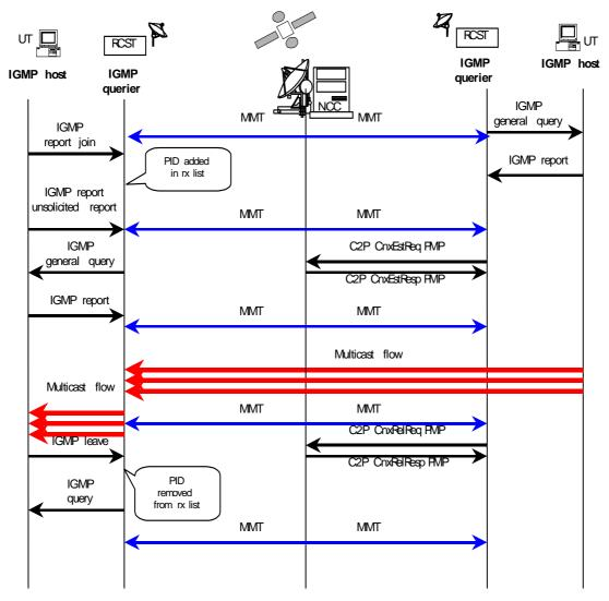
Figure E.2.6: Mesh IP Multicast scenario example
