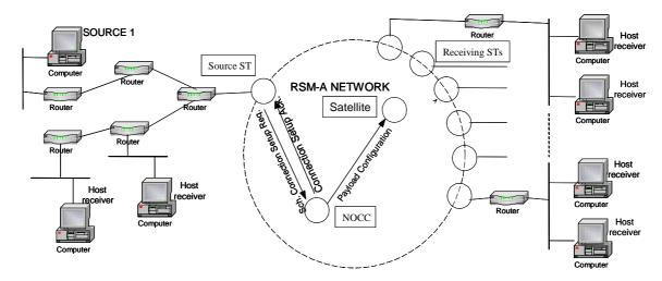
Figure D.3.1 illustrates the Scheduled Multicast Connection Setup process.
