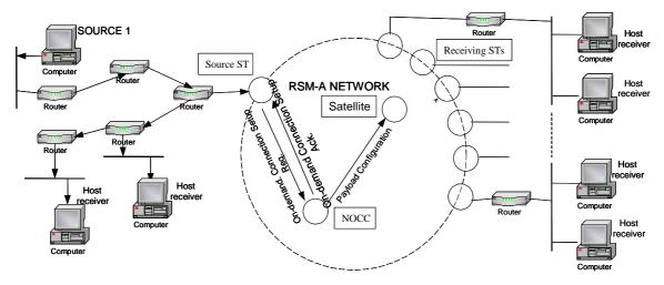
Figure D.4.1: On-demand Multicast Connection Setup
