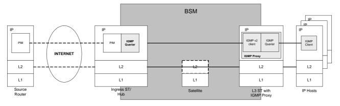
Figure 5.5: IGMP-over-BSM Architecture with Egress ST Layer 3 Forwarding
