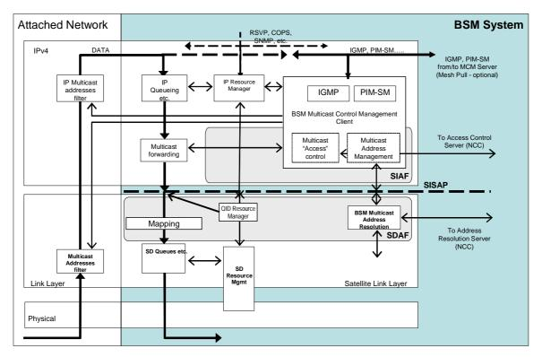
Figure 6.1: BSM Multicast Ingress ST protocol stack
