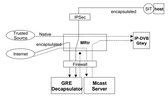
Figure C.5.1: Multicast source transmission model
