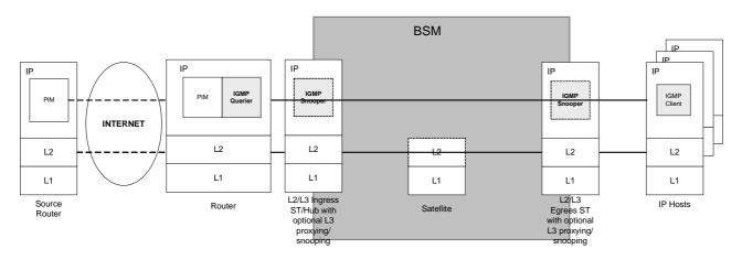
Figure 5.6: IGMP-over-BSM Architecture with IGMP external to BSM and optional IGMP proxying or snooping at Ingress and Egress
