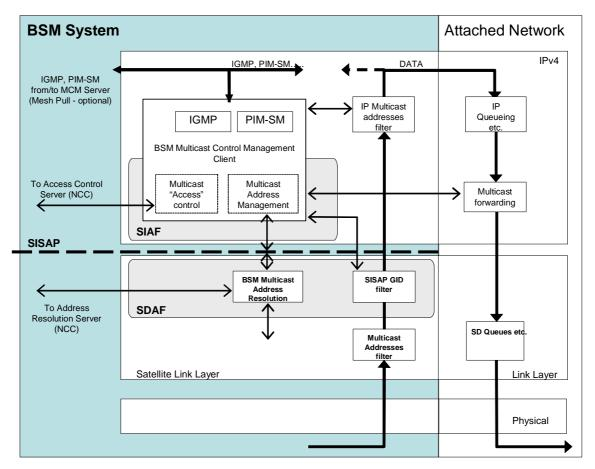
Figure 6.2: BSM Multicast Egress ST protocol stack
