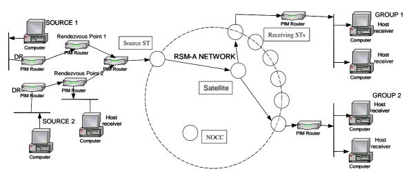
Figure D.5.2: Multicast Datagram Forwarding in RSM-A using PIM-SM STs
