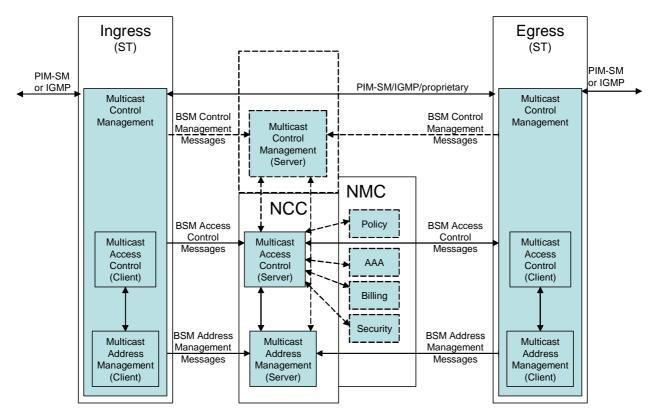
Figure 5.3: BSM Multicast Source Management Control Plane Architecture (Mesh Pull case)
