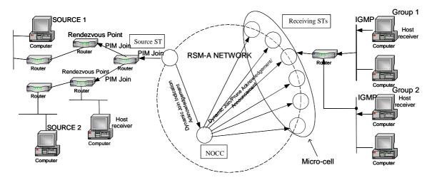
Figure D.4.5: RSM-A Dynamic Join/Prune Acknowledgement
