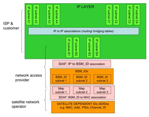
Figure 4.1: BSM Address Management layers
