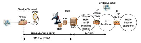
Figure A.9: PPP router access mode with Gateway in LAA mode
