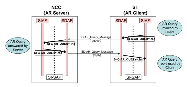
Figure G.2: Example of use of SI-C-AR\_QUERY primitives
