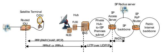
Figure A.6: L2TP Access Aggregation mode
