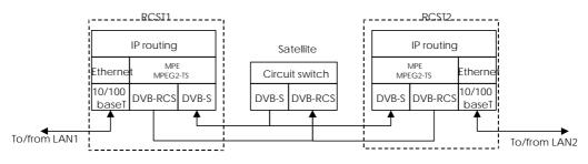
Figure D.3: RCST RSM-B IP routing function
