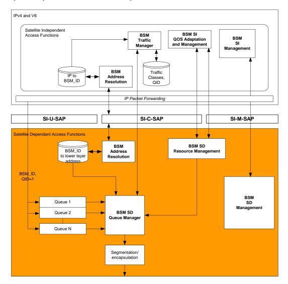
Figure 5.1: BSM protocol stack
