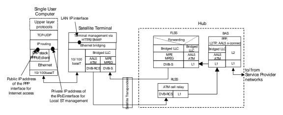
Figure A.4: Protocol stack for the bridged mode
