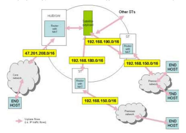
Figure C.1: BSM Network with two Customer Premises Networks
