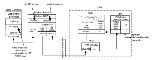
Figure A.10: DHCP router mode protocol stacks
