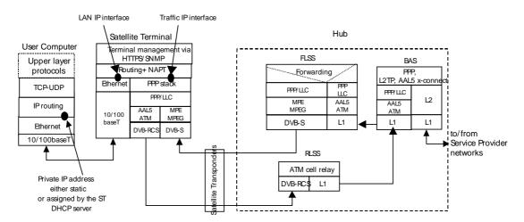
Figure A.7: Protocol stack for PPPoA Router access mode
