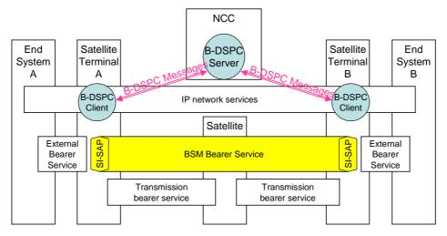
Figure 5.3: BSM B-DSPC Architecture
