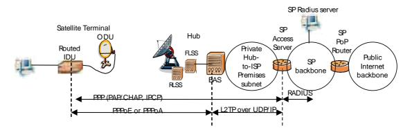
Figure A.8: PPP router access mode with Gateway in PTA mode
