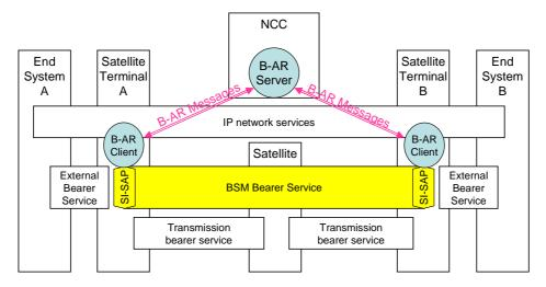
Figure 5.2: BSM AR Architecture
