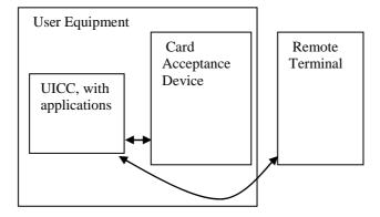
Figure 1: Possible secure channels with a UICC
