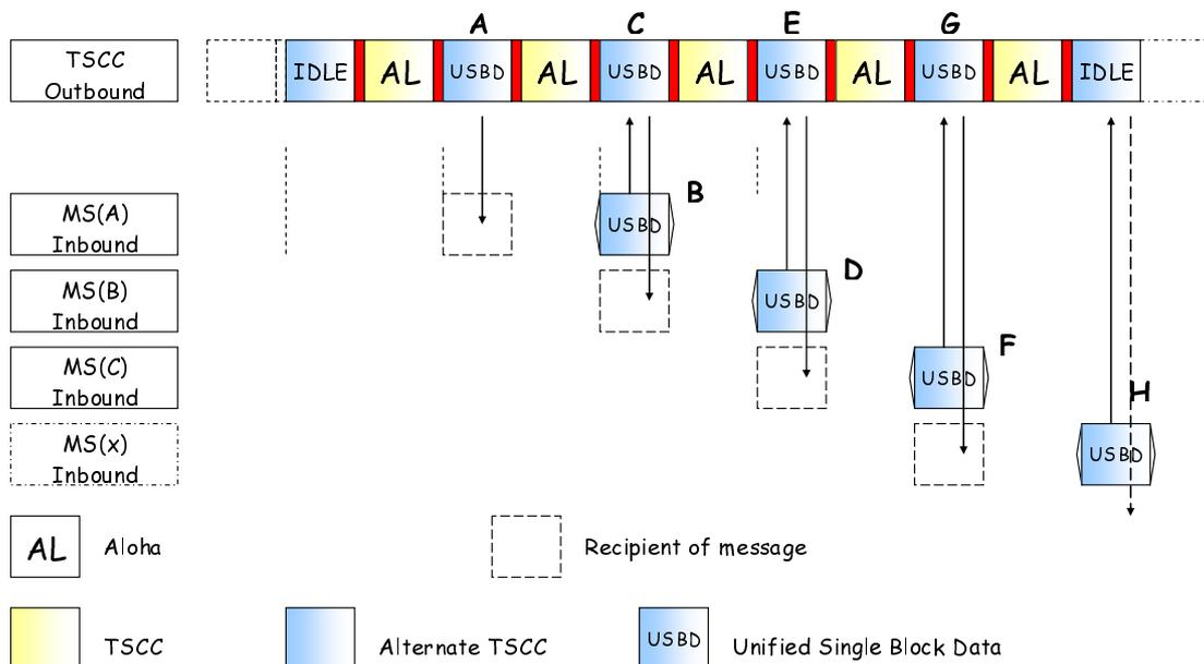
**Figure 6.61: Example of Unified Single Block Data Polling Service on TSCCAS using Aligned Timing (Response Delay=00<sub>2</sub>)**
