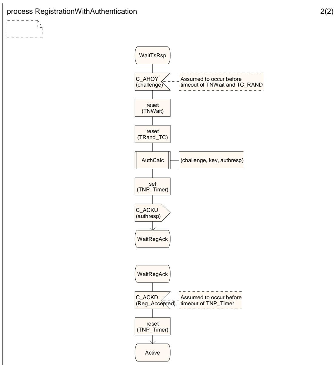
**Figure 6.23 (sheet 2 of 2): Registration with Authentication SDL**
