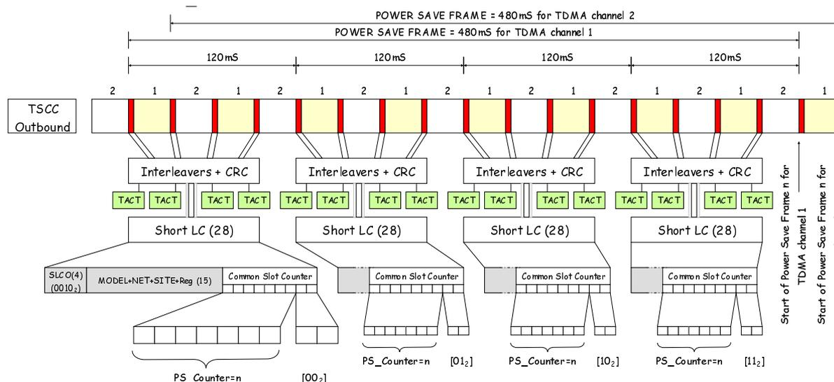
**Figure 6.26: Power Save Frame Structure**
