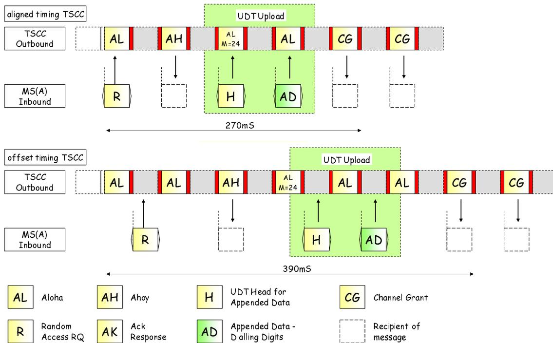
**Figure 6.41: MS to PABX/PSTN Call using the UDT Mechanism**
