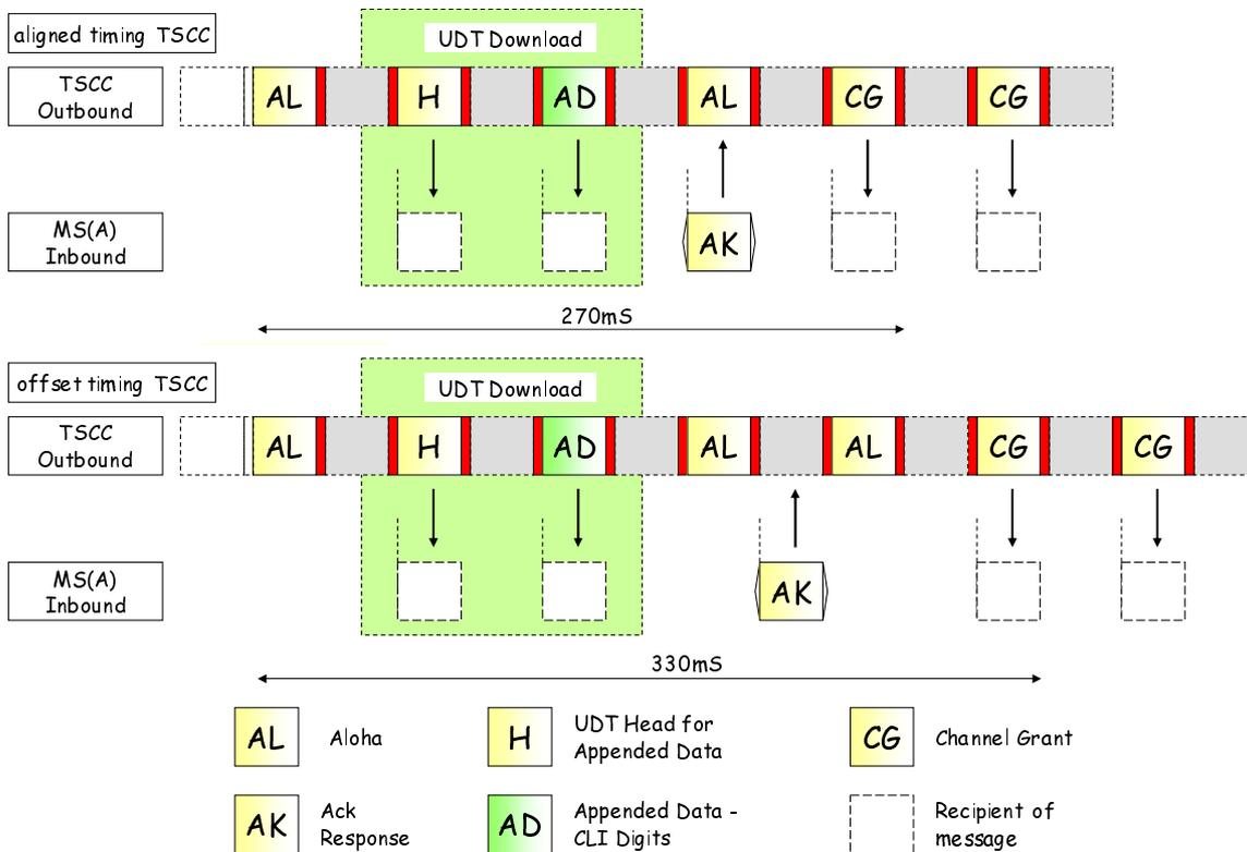
**Figure 6.42: Call from the PSTN/PABX using the UDT Mechanism**
