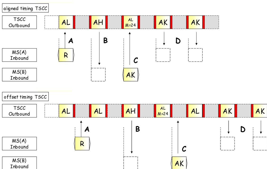
**Figure 6.55: Example of the Status Delivery Service to an individual MS**
