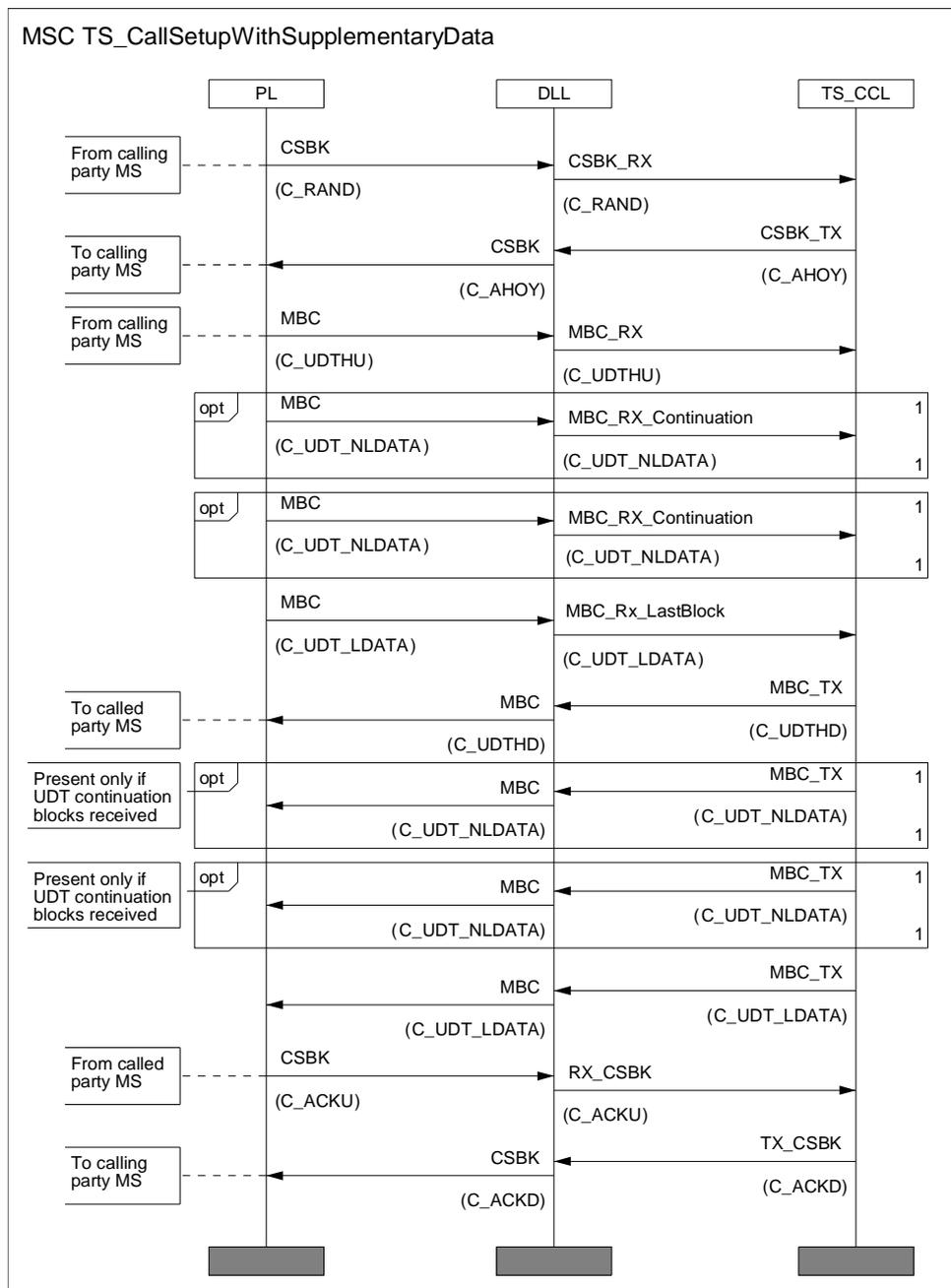
Figure 6.48: MS OACSU Call set-up with Supplementary data
