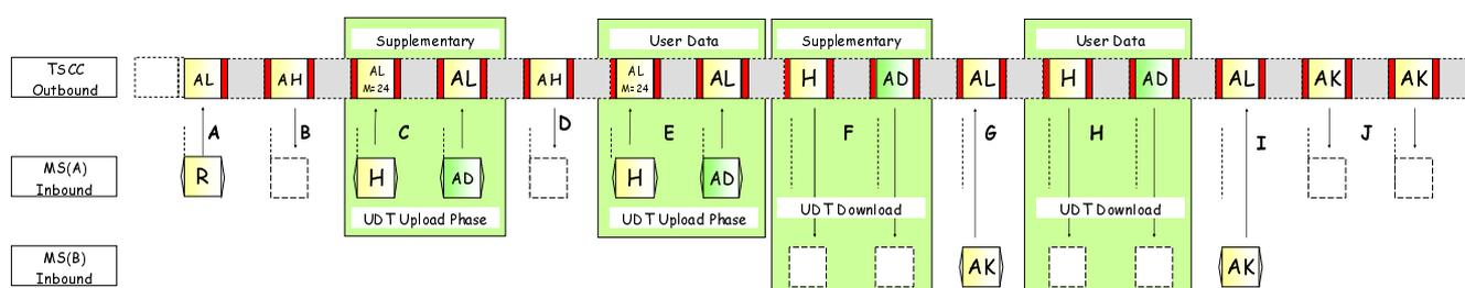
**Figure 6.36: UDT mechanism carrying Supplementary User Data for a UDT Short Data Call**
