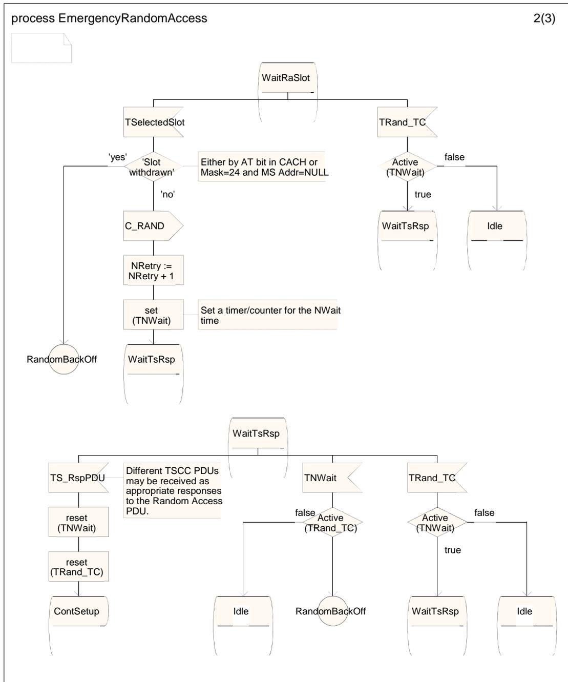
Figure 6.12 (sheet 2 of 3): Emergency Random Access Procedure SDL
