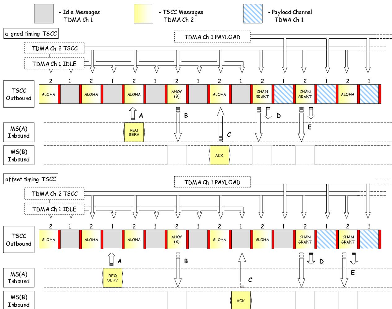
**Figure 4.3: Individual Call Set-up example using OACSU**
