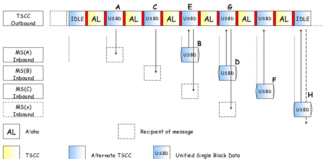
**Figure 6.63: Example of Unified Single Block Data Polling. Response Delay = 90 mS using Aligned Timing (Response Delay =  $01_2$ )**
