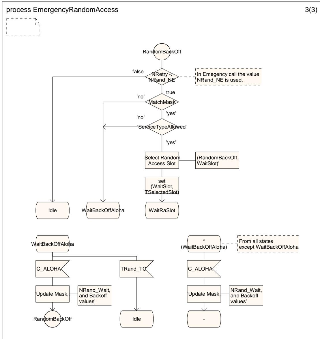
**Figure 6.13 (sheet 3 of 3): Emergency Random Access Procedure SDL**
