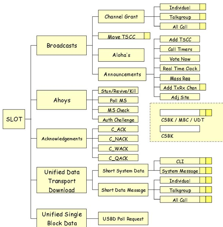
Figure 7.1: Hierarchy for the TSCC outbound channel PDUs
