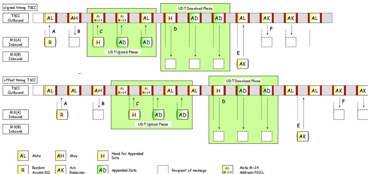
**Figure 6.50: Example of a UDT Short Data Message transfer**
