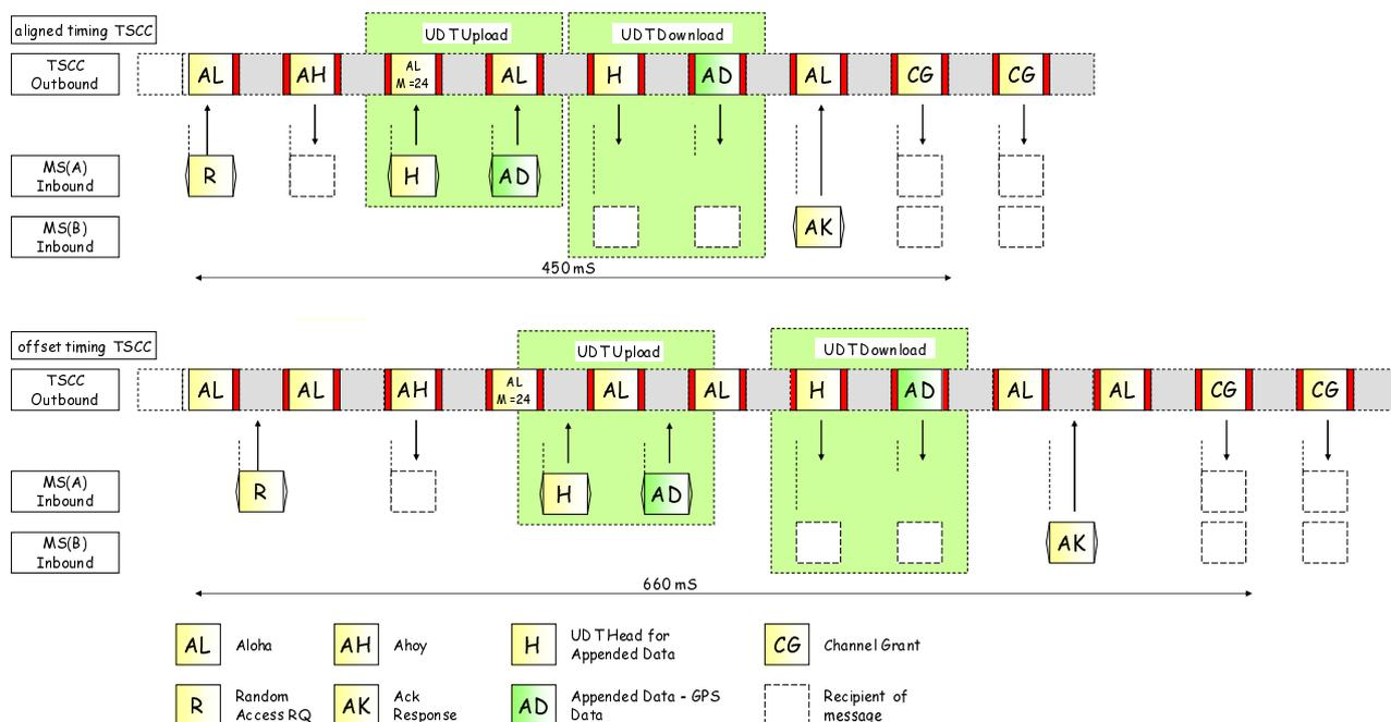
**Figure 6.43: UDT mechanism carrying supplementary data**
