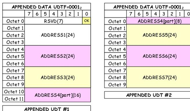
Figure B.7: Appended data Address Format (7 addresses)
