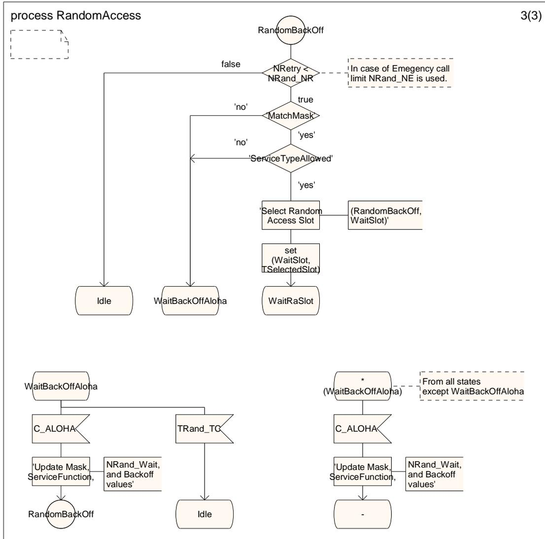
Figure 6.10 (sheet 3 of 3): Random Access Procedure SDL
