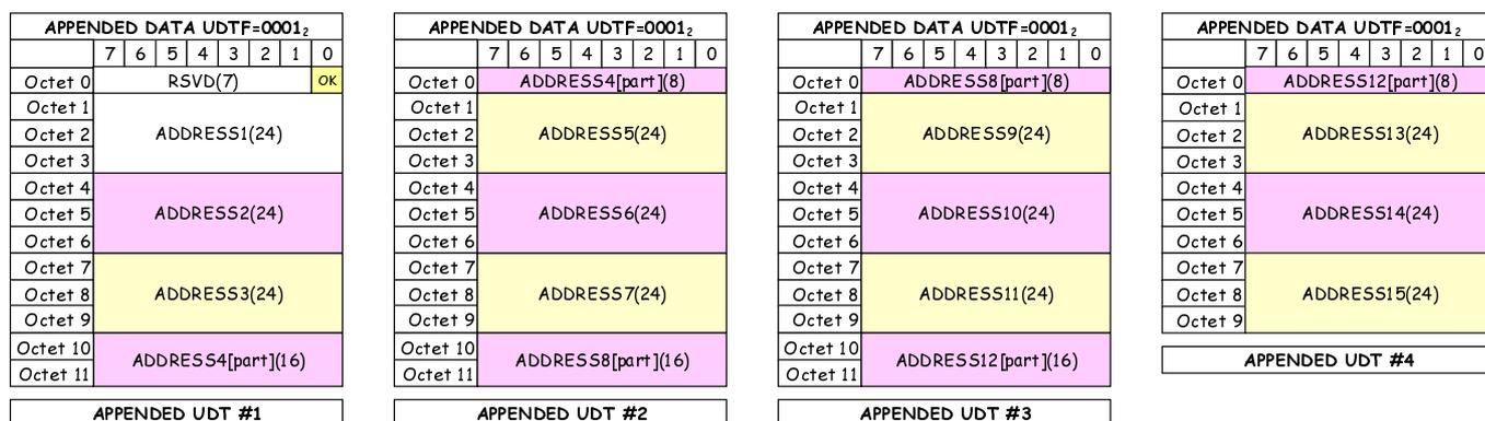
Figure B.9: Appended data Address Format (15 addresses)
