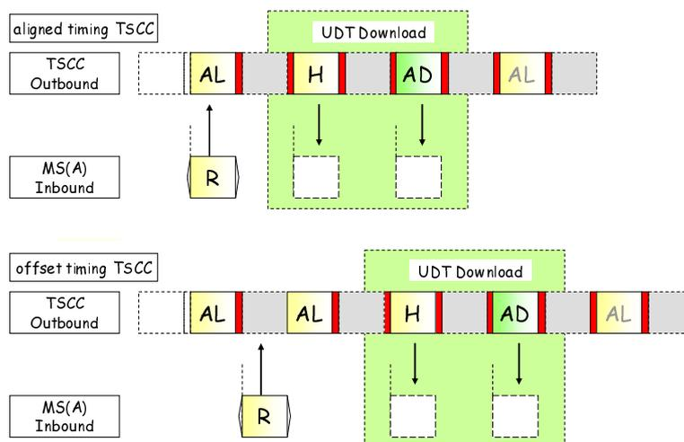
**Figure 6.59: TSCC provides diverted address to MS**
