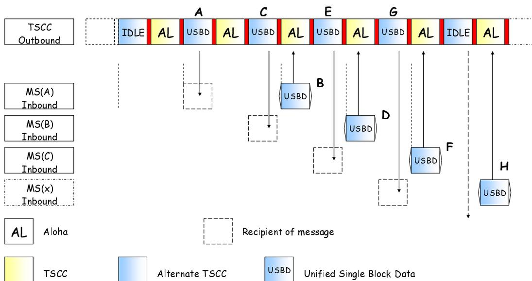
**Figure 6.62: Example of Unified Single Block Data Polling Service on TSCCAS using Offset Timing (Response Delay =  $00_2$ )**
