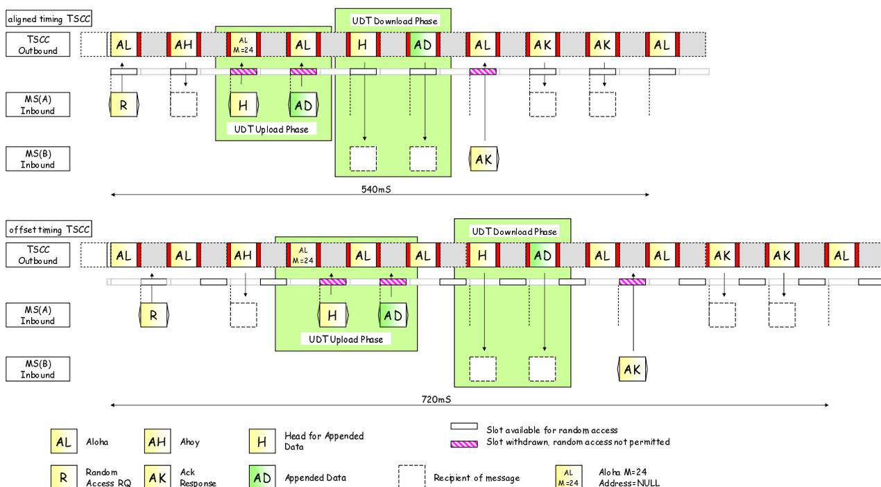
Figure 6.40: A UDT Short Data call using the UDT mechanism
