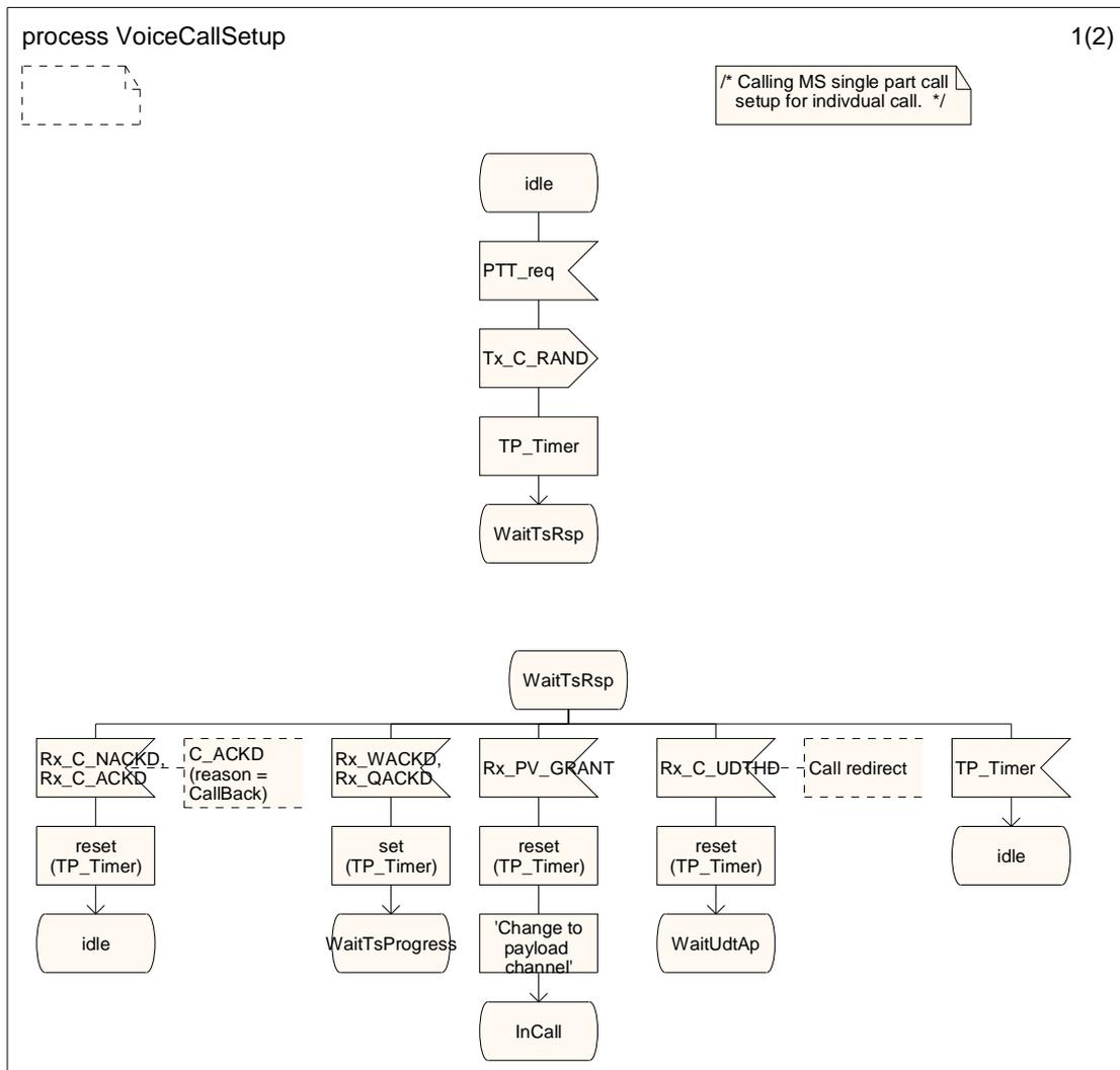
Figure 6.46 (sheet 1 of 2): Single part OACSU voice call setup SDL
