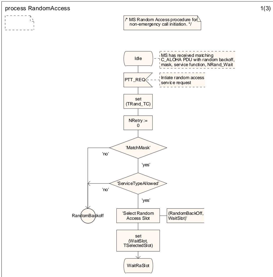
Figure 6.8 (sheet 1 of 3): Random Access Procedure SDL
