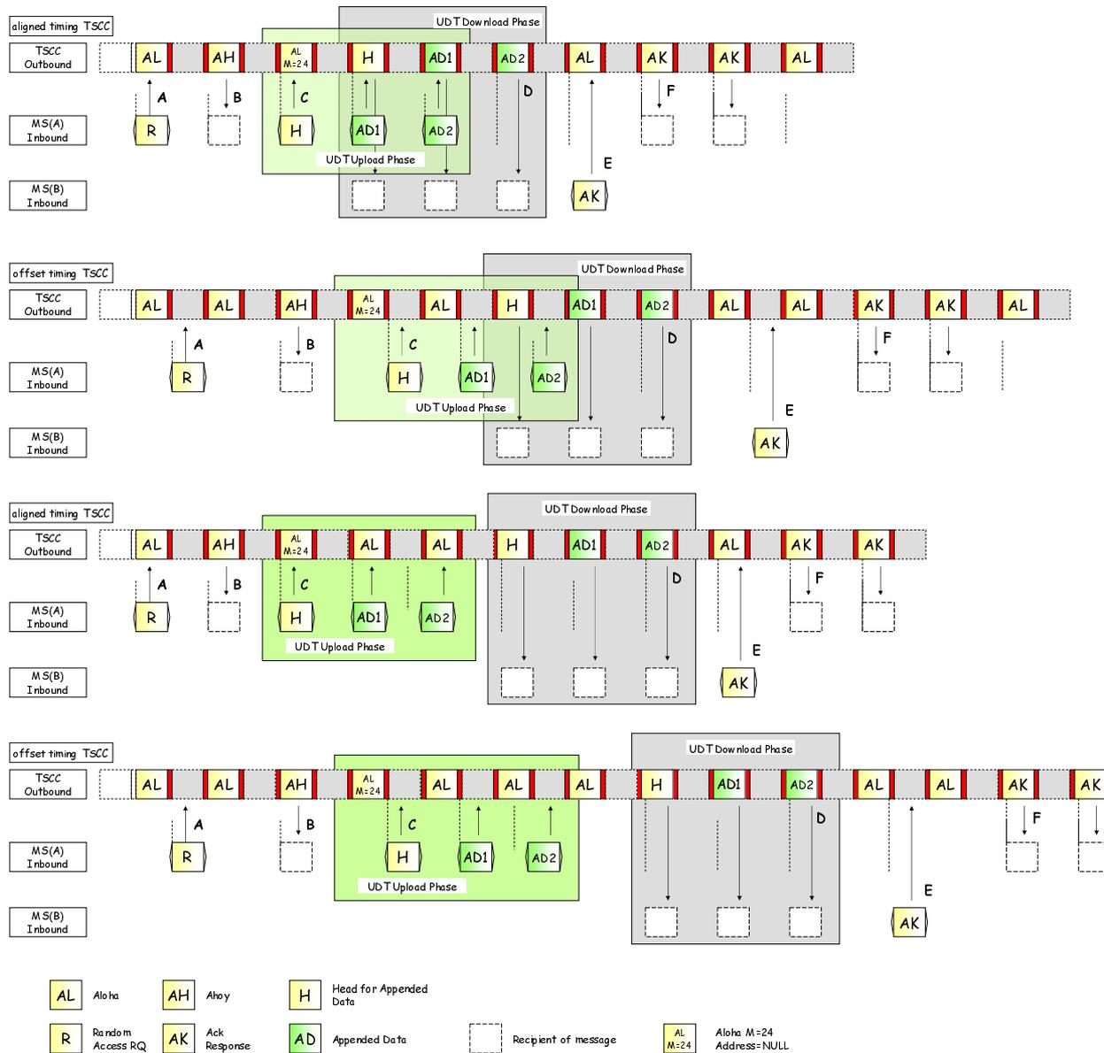
Figure 6.51: More Examples of a UDT Short Data Message transfer
