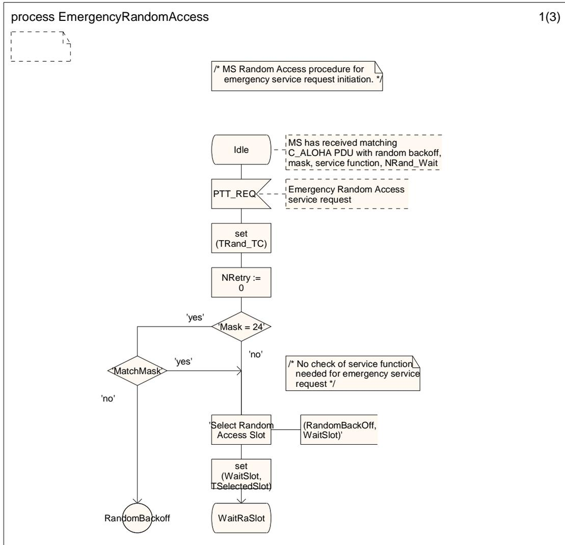
Figure 6.11 (sheet 1 of 3): Emergency Random Access Procedure SDL
