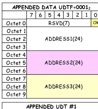
Figure B.6: Appended data Address Format (3 addresses)
