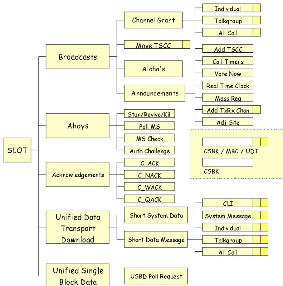
Figure 5.3: TSCC CSBK/MBC/UDT/USB D Outbound Channel Structure
