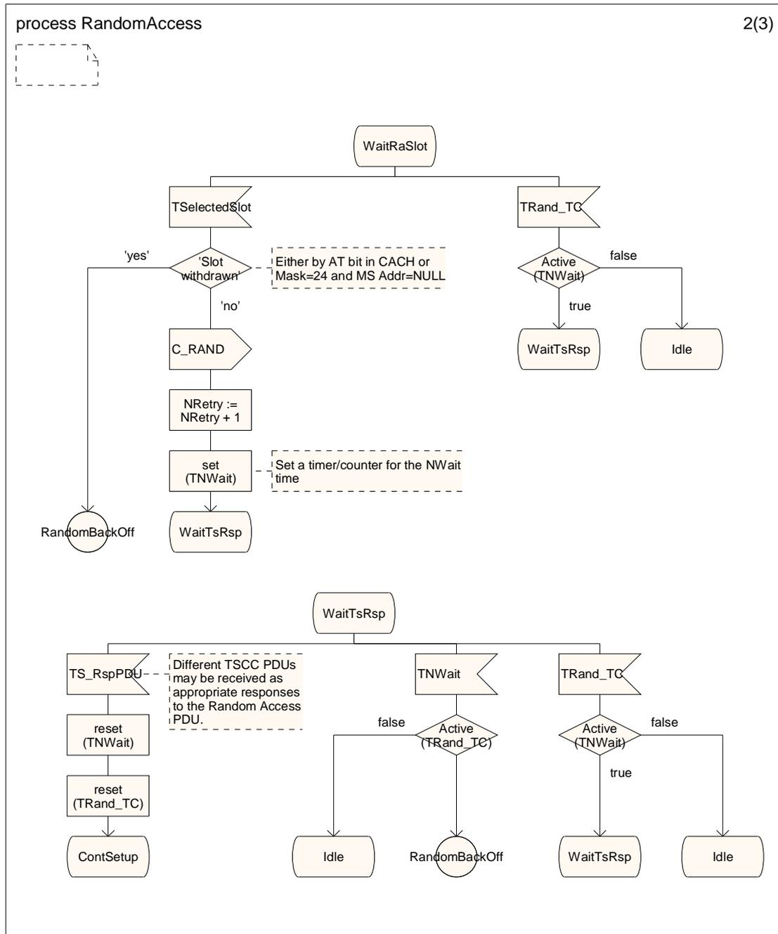
Figure 6.9 (sheet 2 of 3): Random Access Procedure SDL
