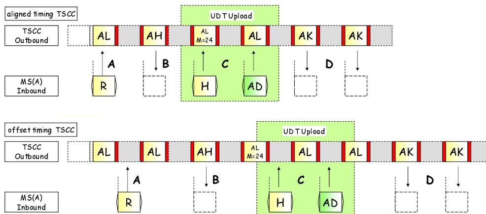
**Figure 6.44: Example of Multi-part call procedure**
