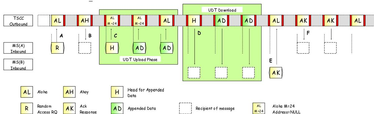
**Figure 6.60: Example of a Dynamic Group Numbering Assignment transfer**
