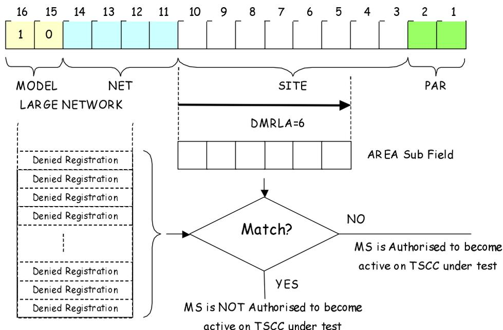
**Figure 6.18: SYS\_AREA information element from the C\_SYSCode**
