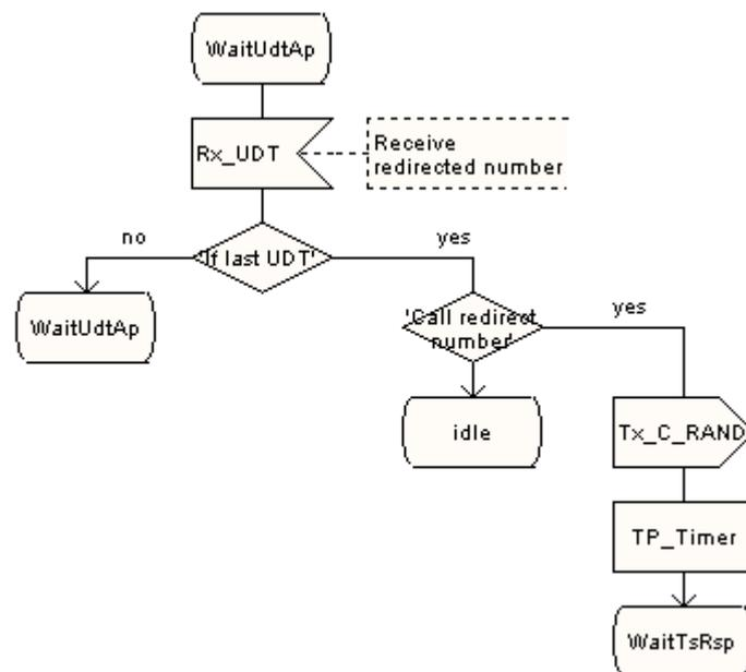
Figure 6.47 (sheet 2 of 2): Single part OACSU voice call setup SDL
