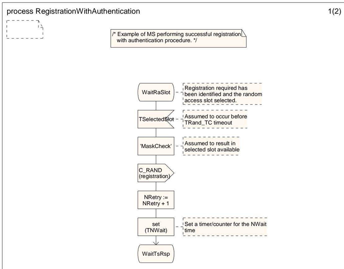
Figure 6.22 (sheet 1 of 2): Registration with Authentication SDL
