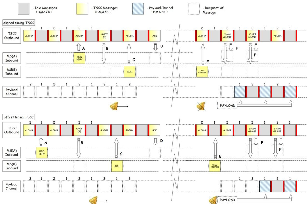
**Figure 4.4: Individual Call Set-up example using FOACSU**
