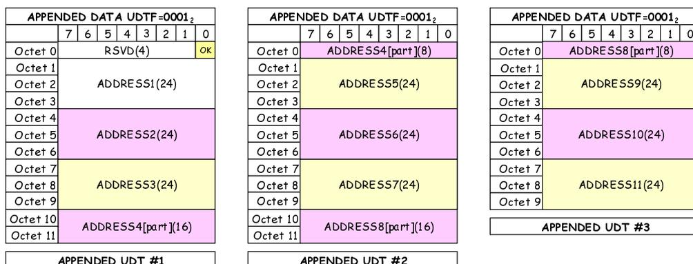
Figure B.8: Appended data Address Format (11 addresses)
