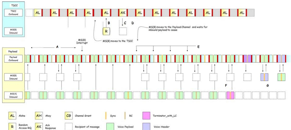
**Figure 6.37: Payload Interrupt MS De-key**
