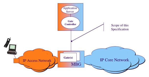
Figure 3: Example of Gate Control architecture for non-conversational service
