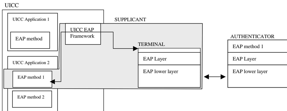
Figure 4.1: EAP architecture when supplicant is split between a UICC and a terminal
