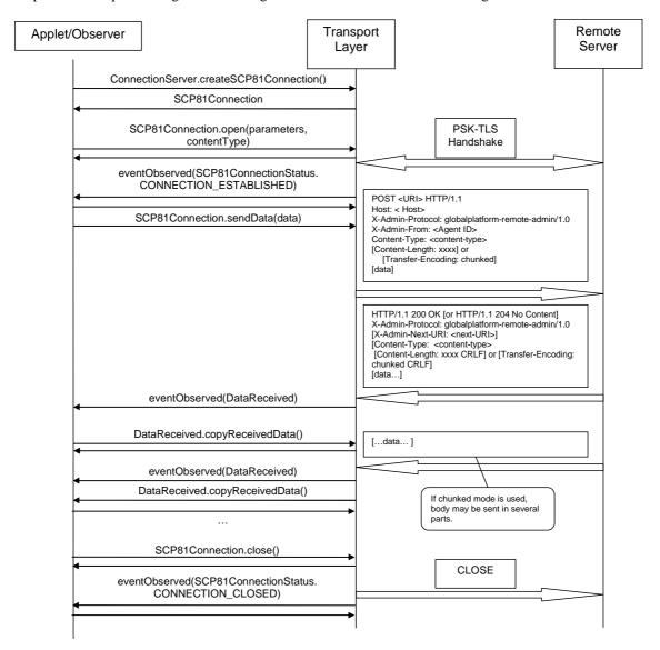
Figure 5: SCP81Connection sequence diagram
