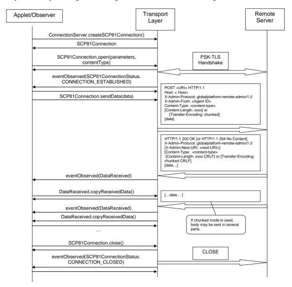
Figure 5: SCP81Connection sequence diagram
