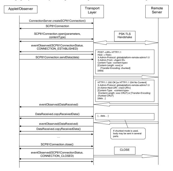
Figure 5: SCP81Connection sequence diagram
