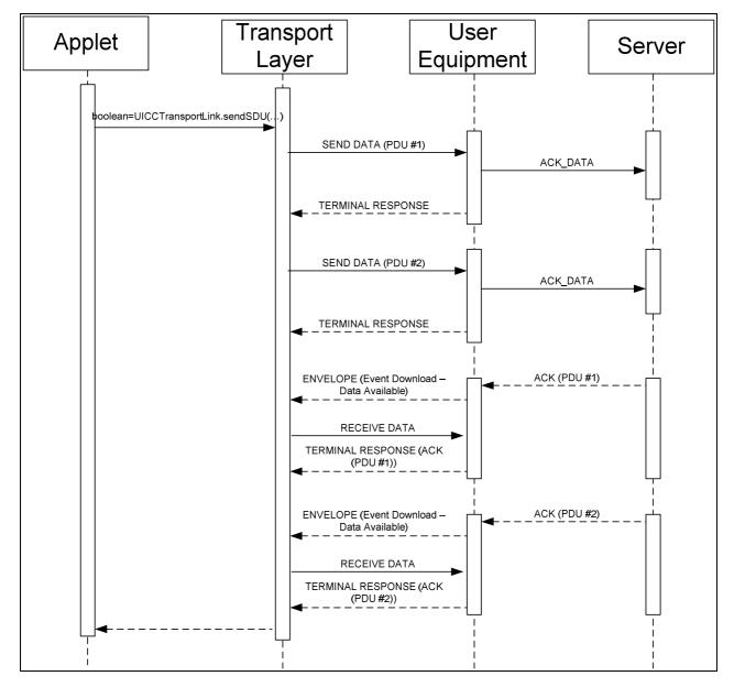
Figure 3: Sending data over Reliable Link
