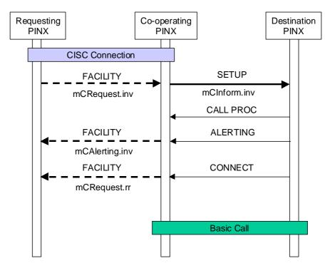
Figure B.2: Example of successful invocation and operation of SS-MCR using an already existing CISC
