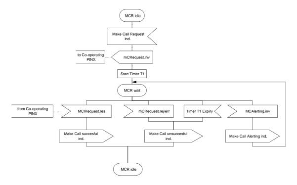
Figure C.1: SDL representation of SS-MCR at the Requesting PINX
