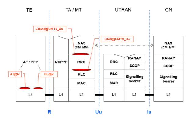
Figure 7.5: 3G CS domain and PS control plane
