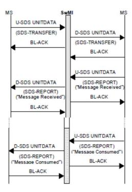
Figure 70: SDS signalling flow chart
