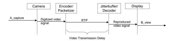
Figure 54: The Video Transmission Delay
