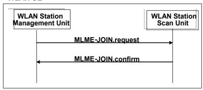
Figure 37: JOIN Signal Flow
