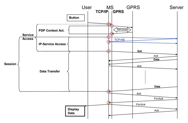
Figure 3: QoS parameters version B (Example: HTTP via GPRS)
