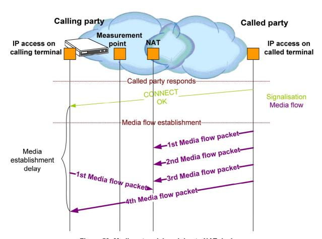
Figure 59: Media setup delayed due to NAT devices
