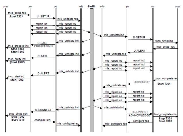
Figure 27: Individual call set-up using on/off hook signalling (ETSI EN 300 392-2 [27], clause 14.5.1)
