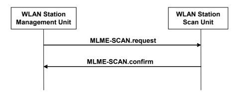
Figure 35: SCAN Signal Flow
