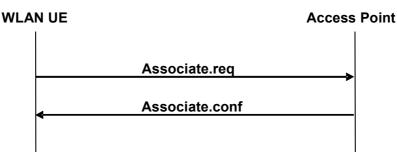
Figure 43: WLAN RE-ASSOCIATION Signal Flow
