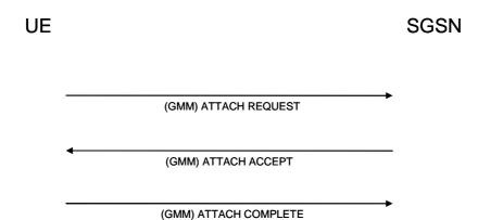
Figure 4: GPRS/UMTS attach procedure
