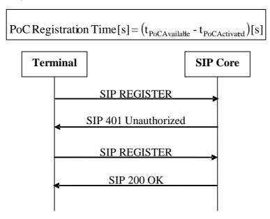
NOTE: This figure shows an example of a successful PoC registration (see [16]). In contrast to Figure 13, the terminal answered correctly to the authentication challenge (the second "SIP REGISTER" message).
