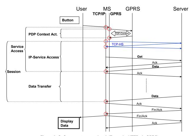
Figure 2: QoS parameters version A (Example: HTTP via GPRS)
