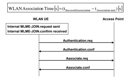
Figure 42: WLAN ASSOCIATION Signal Flow
