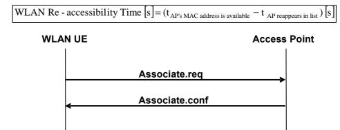
Figure 44: WLAN RE-ASSOCIATION Signal Flow
