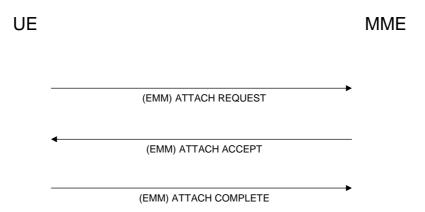
Figure 5: LTE attach procedure
