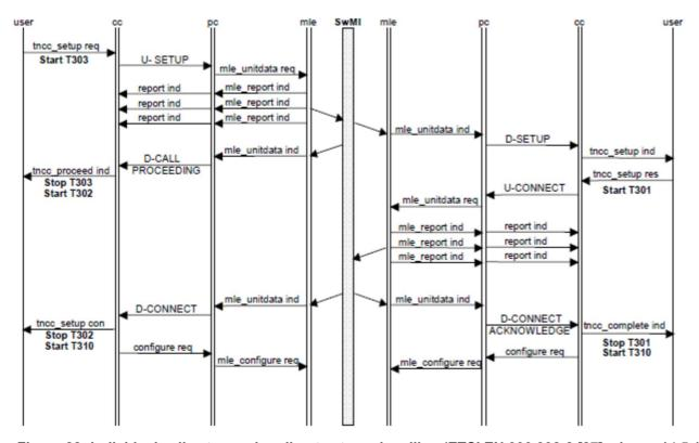
Figure 28: Individual call set-up using direct set-up signalling (ETSI EN 300 392-2 [27], clause 14.5.1)
