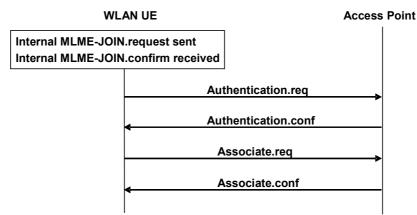
Figure 41: WLAN ASSOCIATION Signal Flow
