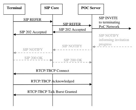
NOTE: The dashed arrows in this figure only occur in case of a confirmed, manual answer invitation. In this case the time period between the "SIP INVITE" message and the reception of the "Talk Burst Granted" message depends on how fast an invited user on the terminating side answers to the invitation. Furthermore, the "SIP NOTIFY" message is defined as optional (see [15]) and might not be sent by the server at all. For this reason the automatic answer mode shall be used during measurements.
