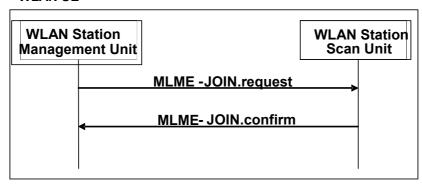
Figure 39: JOIN Signal Flow
