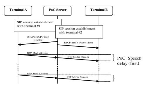
Figure 22: PoC speech transmission delay (first) and PoC speech transmission delay (others)
