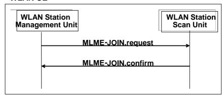
Figure 29: JOIN Signal Flow
