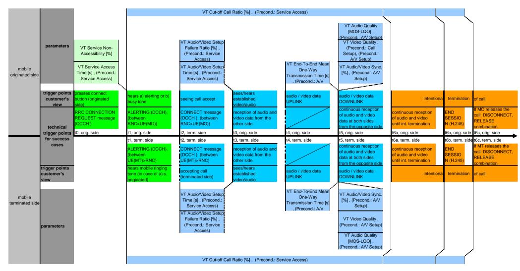
Figure 24: Parameter overview with trigger points
