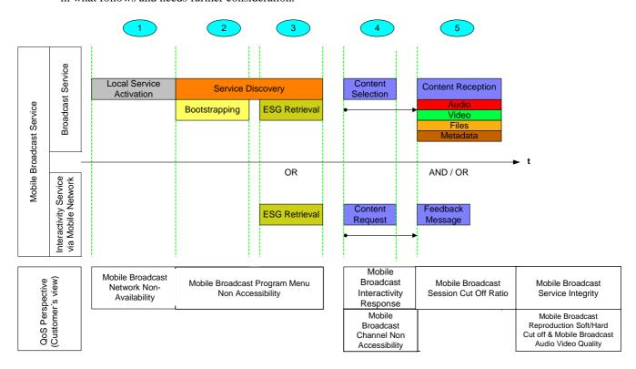
Figure 4: Service phases of mobile broadcast
