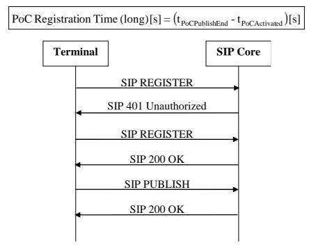
Figure 9: Example for a successful PoC Registration (long)
