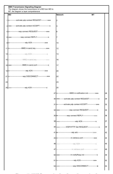
Figure 42: MMS Transaction flow (immediate retrieval)
