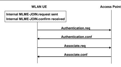
Figure 33: WLAN ASSOCIATION Signal Flow
