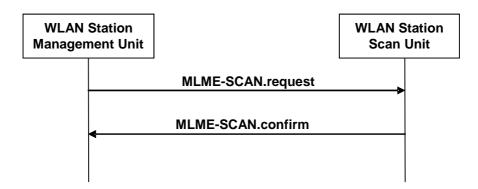
Figure 27: SCAN Signal Flow
