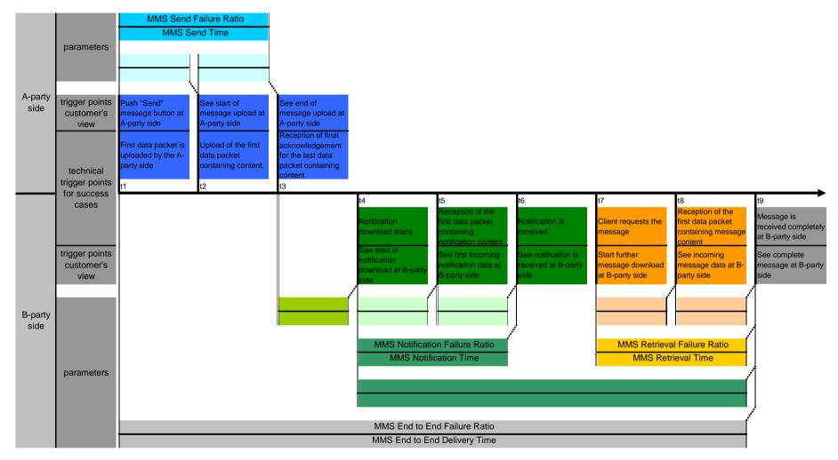
Figure 41: MMS Parameter Overview with Trigger Points
