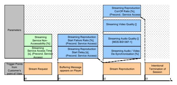
Figure 22: Parameter overview with trigger points
