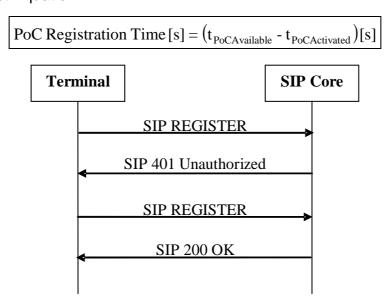
NOTE: Figure 7 shows an example of a successful PoC registration (see [16]). In contrast to figure 11, the terminal answered correctly to the authentication challenge (the second "SIP REGISTER" message).
