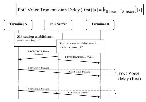
Figure 20: PoC voice transmission delay (first) and PoC voice transmission delay (others)
