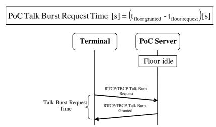
Figure 18: Example for a successful talk burst request
