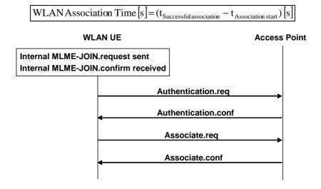
Figure 34: WLAN ASSOCIATION Signal Flow
