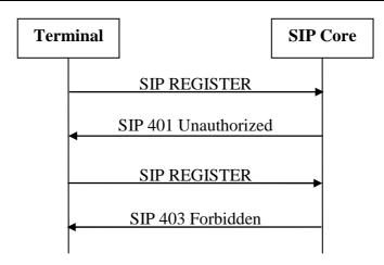
NOTE: Figure 6 shows an example for an unsuccessful PoC registration. After the first "SIP REGISTER" request the terminal has to answer to a WWW- authentication challenge (see [16]). If the terminal does not answer correctly to this challenge, the SIP core will send a "SIP 403 Forbidden" message.
