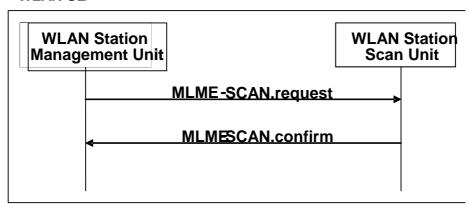
Figure 28: SCAN Signal Flow
