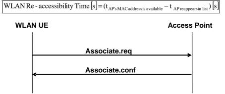
Figure 36: WLAN RE-ASSOCIATION Signal Flow
