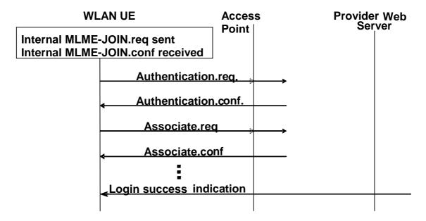
Figure 30: WLAN PS Data Service Provisioning Signal Flow
