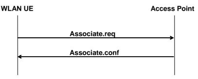
Figure 35: WLAN RE-ASSOCIATION Signal Flow
