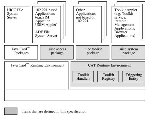
Figure 1: UICC Java Card™ architecture
