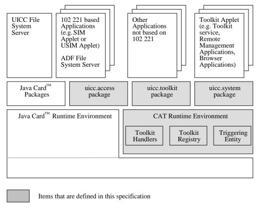
Figure 1: UICC Java Card™ architecture
