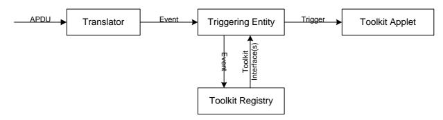
Figure 3: toolkit applet triggering diagram
