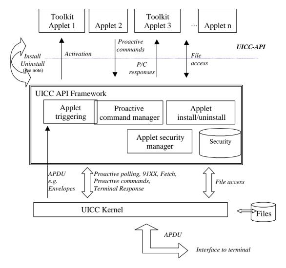
NOTE: The install/uninstall process does not form part of the API. Its requirements are outlined in clause 7.
