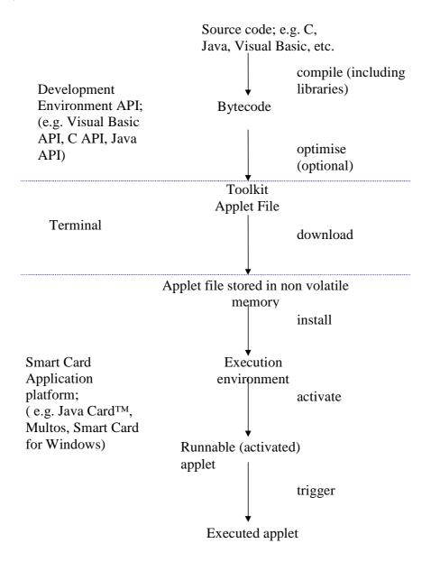
Figure 2: Flow diagram of the development of a UICC application
