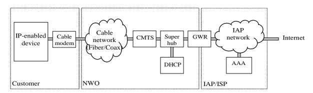
Figure 4: Cable modem access
