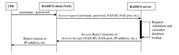
Figure A.3: Basic authentication message exchange
