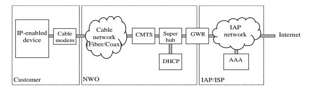
Figure 4: Cable modem access
