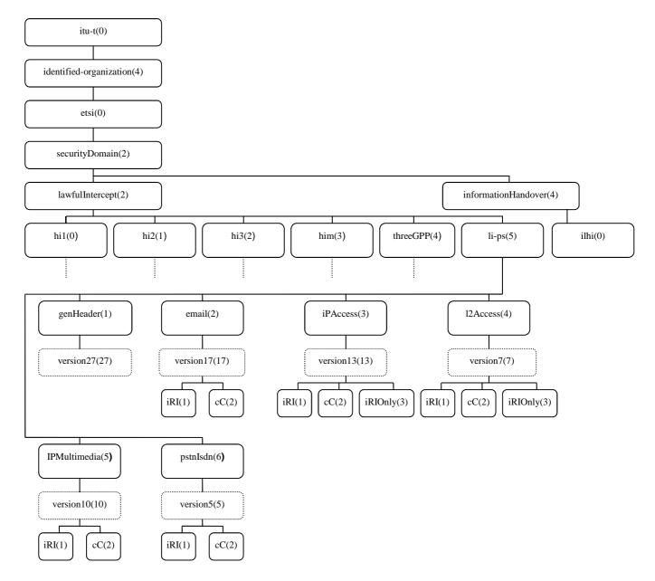
Figure A.1: Object identifier tree
