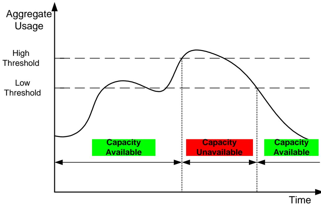
Figure 2: Example of capacity Available/Unavailable transitions
